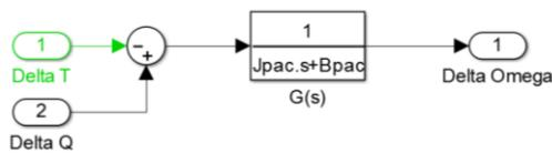
Figure 180: Simulink Model -  $\Delta\omega$  Estimator
