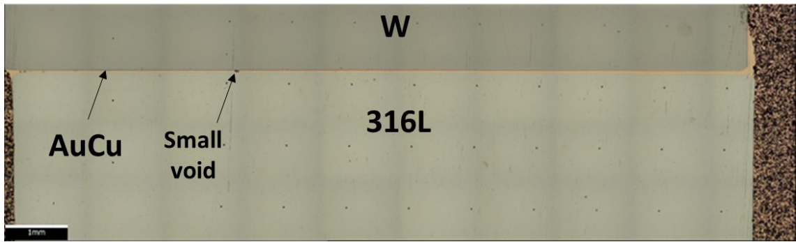
Figure 3-22 - W-AuCu-316L brazed interface - entire cross section
