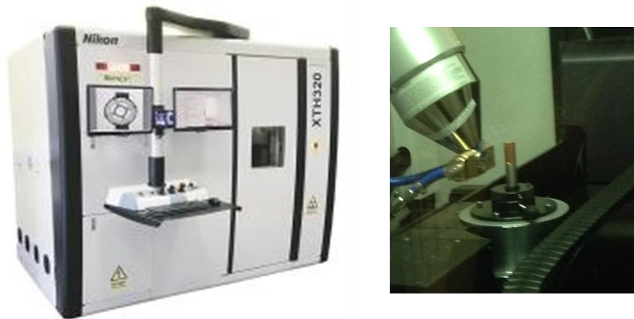
Figure 3-51 - XCT equipment and W-AuCu-Cu brazed sample positioned for evaluation
