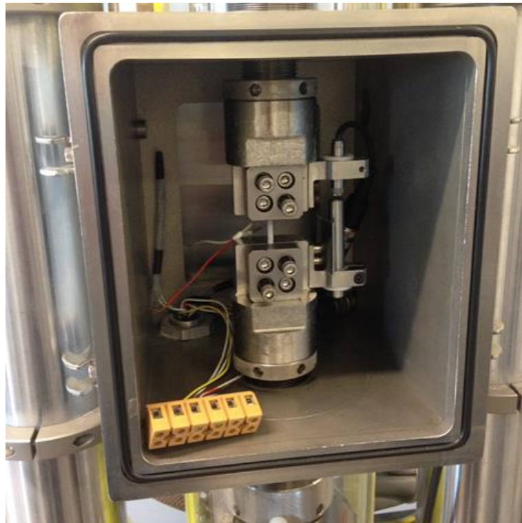
Figure 4-29 - ETMT set-up with Au80Cu20 specimen installed in between grips
