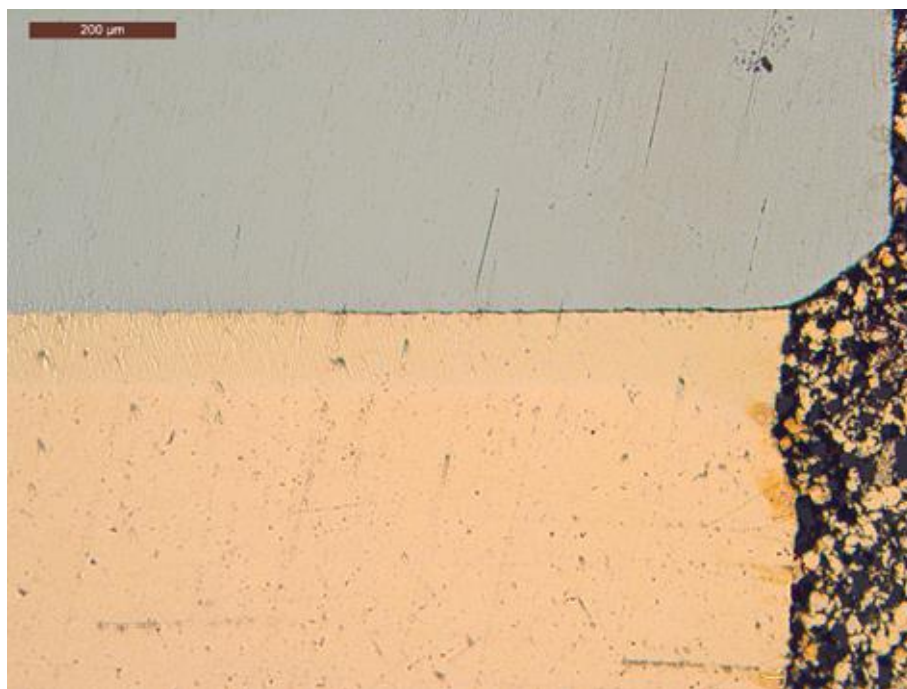
Figure 3-18 – Optical microscope image of W-AuCu-Cu brazed interface - free edge location
