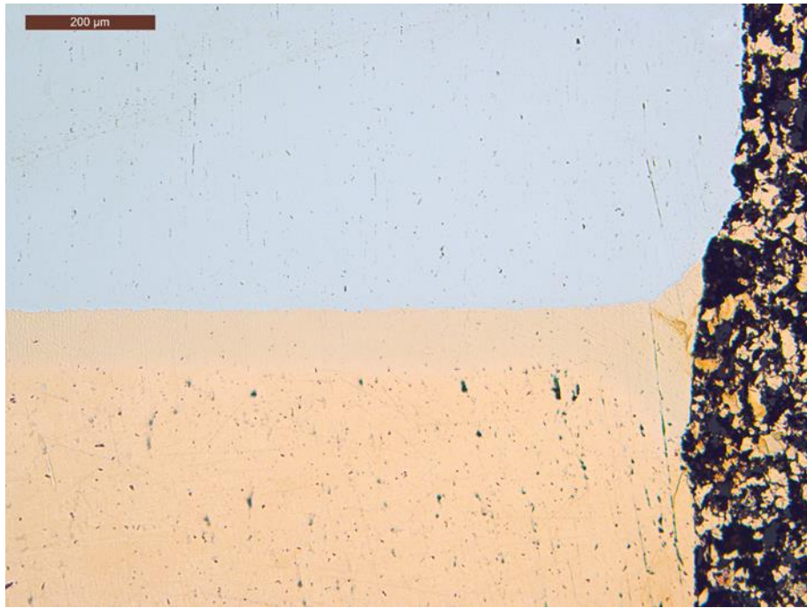
Figure 3-31 - Optical microscope image of 316L-AuCu-Cu brazed interface - free edge location
