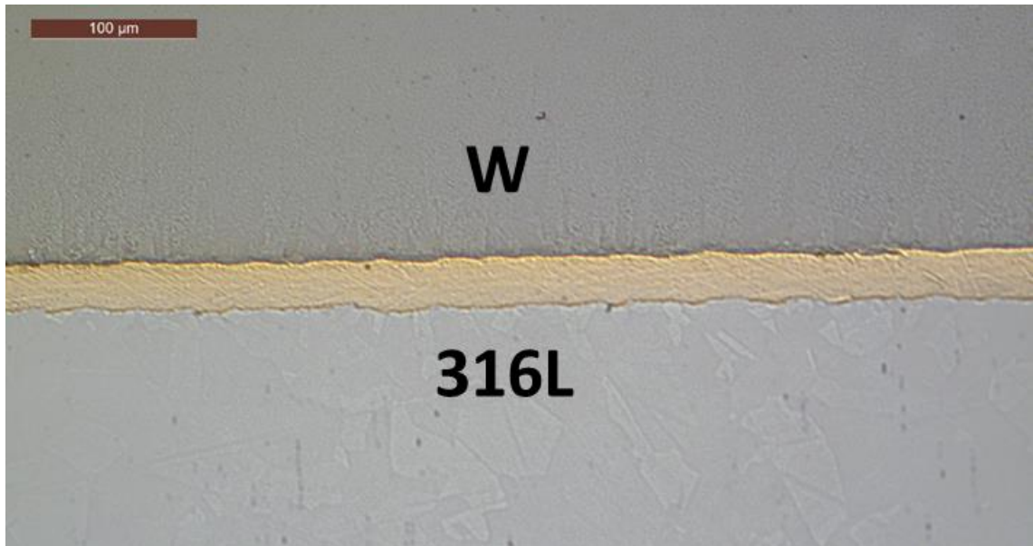
Figure 3-23 - Microstructure of W-AuCu-316L brazed joint
