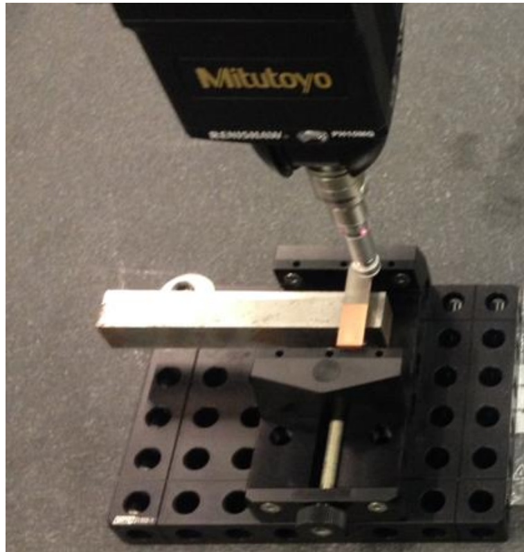
Figure 6-32 - CMM surface measurement of W-AuCu-Cu brazed part for Contour Method residual stress analysis
