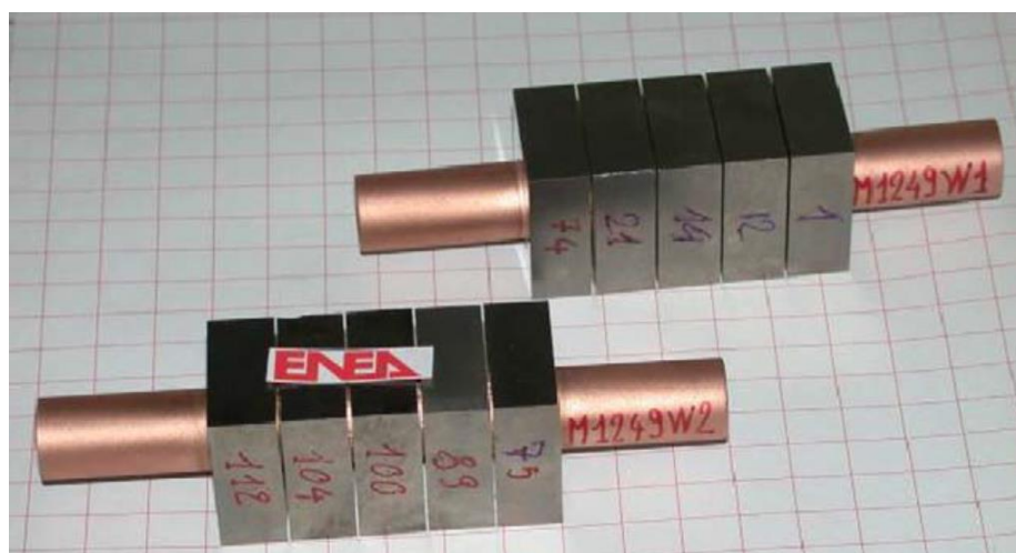
Figure 2-5 - ITER divertor mock-up for HHF testing with tungsten monoblock and CuCrZr heat sink pipe
