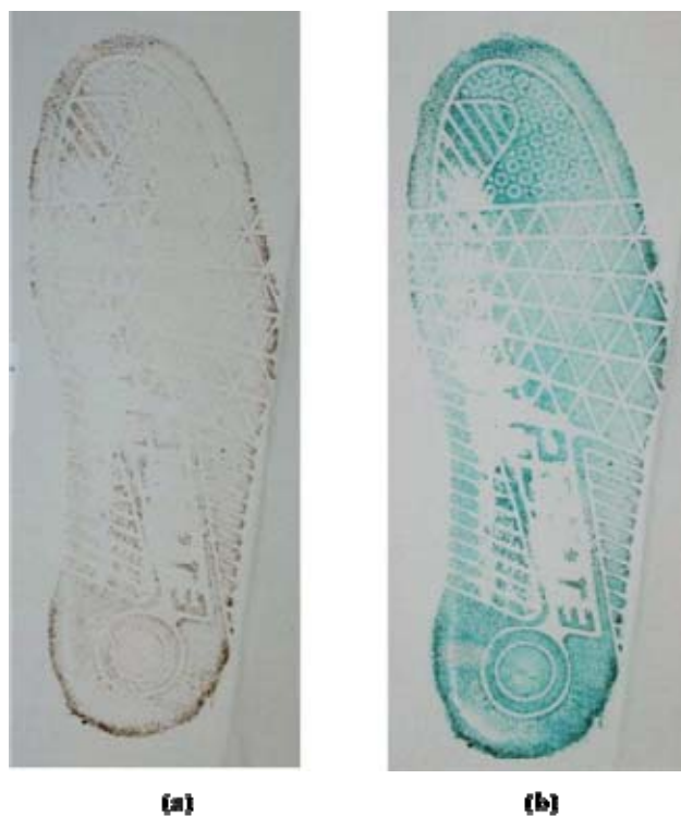
Figure 3.36 - Enhancement of a footwear impression in blood on white cotton using LMG: (a) before; (b) after
