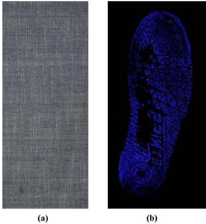
Figure 3.45 - Enhancement of a footwear impression in blood on denim using luminol: (a) before; (b) after
