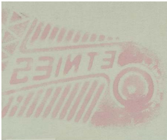
Figure 4.10 - Preliminary DFO enhancement of a footwear impression in urine on white cotton fabric
