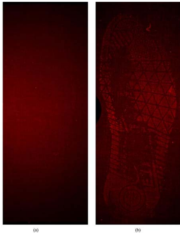
Figure 3.34 - Enhancement of a footwear impression in blood on denim and enhanced with LCV using: (a) Quaser 40 yellow/green excitation source (503-591nm) and (b) yellow laser (577nm)
