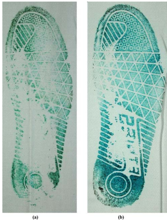
Figure 3.35 - Enhancement of a footwear impression in blood on white cotton using LMG: (a) with fix; (b) without fix
