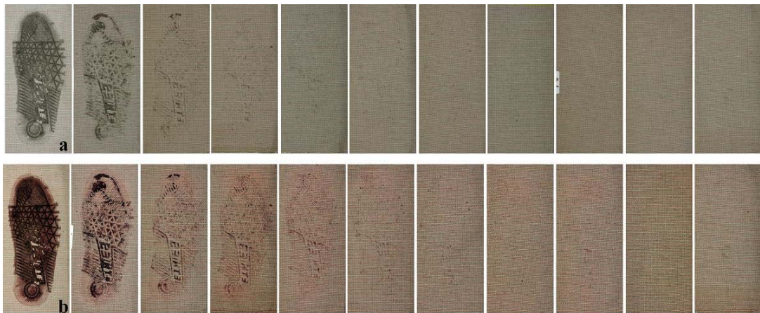
Figure 5.42 - Chemical enhancement of a diminishing series of footwear impressions in mud, prepared with road soil sample on patterned cotton, with potassium thiocyanate: (a) before; and (b) after enhancement
