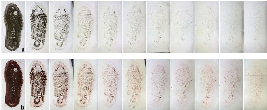
Figure 5.33 - Chemical enhancement of a diminishing series of footwear impressions in mud, prepared with Cornalees soil on white cotton, with potassium thiocyanate: before; and (b) after enhancement
