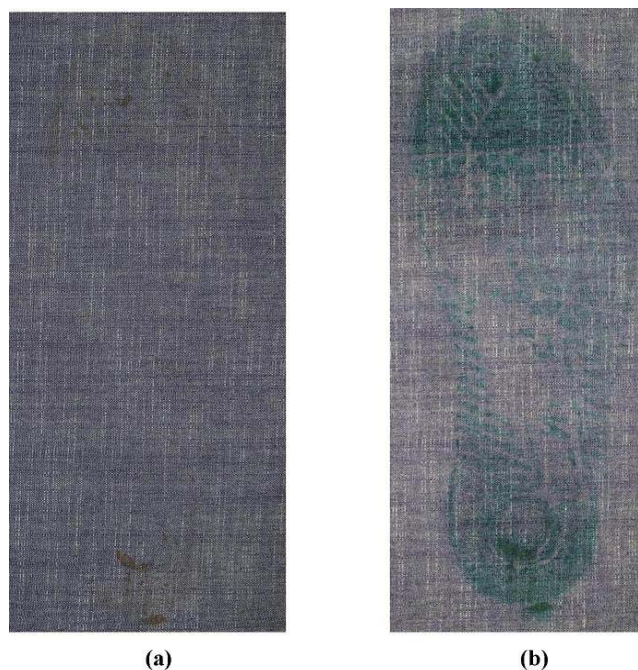
Figure 3.37 - Enhancement of a footwear impression in blood on denim using LMG: (a) before; (b) after
