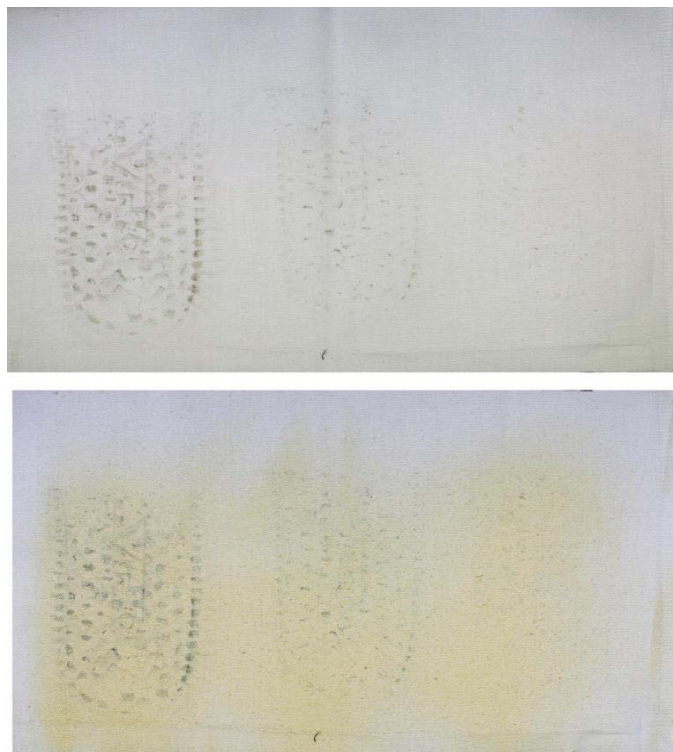
Figure 5.16 - Enhancement of muddy footwear impressions on white cotton for the detection of aluminium: (top) before enhancement; (bottom) after enhancement
