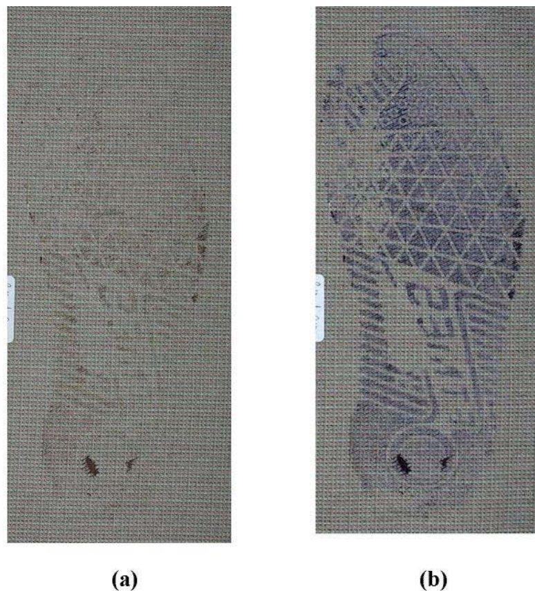
Figure 3.32 – Enhancement of a footwear impression in blood on patterned cotton using LCV: (a) before; (b) after
