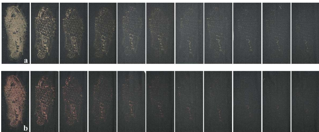
Figure 5.45 - Chemical enhancement of a diminishing series of footwear impressions in mud, prepared with road soil sample on black nylon/lycra, with 2,2'-dipyridil: (a) before; and (b) after enhancement
