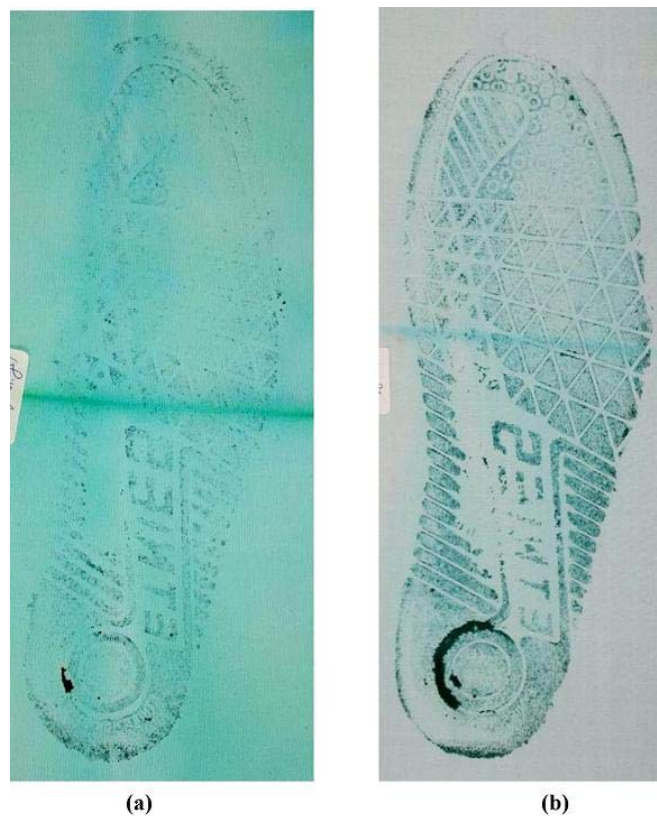
Figure 3.23 - Enhancement of a footwear impression in blood with ABLu1: (a) white cotton; (b) white nylon/lycra
