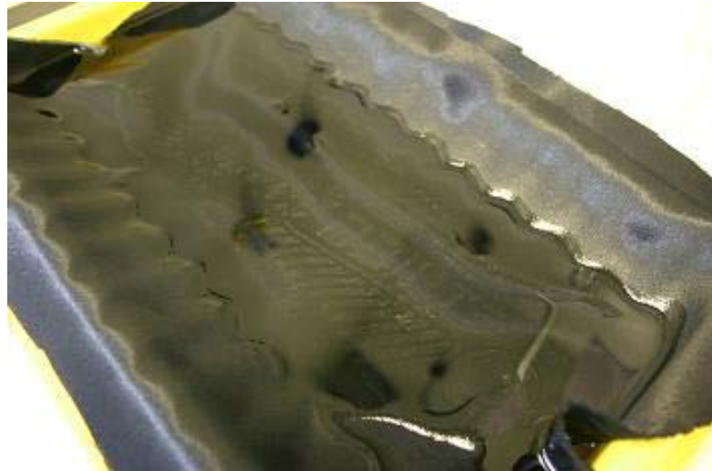
Figure 3.22 - Visualisation of a footwear impression in blood on black polyester during fixation
