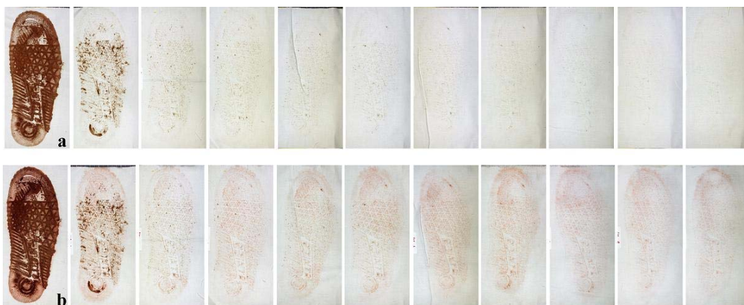
Figure 5.30 - Chemical enhancement of a diminishing series of footwear impressions in mud, prepared with Wemyss Bay soil on white cotton, with PHS: (a) before; and (b) after enhancement
