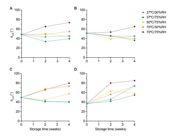
Figure E.12: The change in initial contact angle  $(\theta_{c,0})$  for DCPA/lactose-based tablets with (A) CCS, (B) XPVP, (C) L-HPC and (D) SSG after storage under accelerated storage conditions for 2 and 4 weeks. Mean, n = 2.
