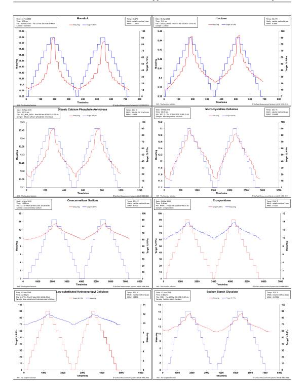
Figure D.1: Settling plots from the dynamic vapour sorption measurements of each filler and disintegrant.
