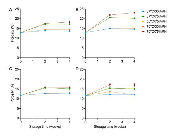
Figure E.5: The change in porosity for MCC/lactose-based tablets with (A) CCS, (B) XPVP, (C) L-HPC and (D) SSG after storage under accelerated storage conditions for 2 and 4 weeks. Mean  $\pm$  standard deviation, n = 100 (0 weeks) and n = 10 (2 and 4 weeks).
