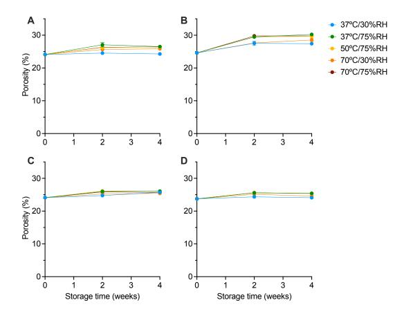
Figure E.7: The change in porosity for MCC/DCPA-based tablets with (A) CCS, (B) XPVP, (C) L-HPC and (D) SSG after storage under accelerated storage conditions for 2 and 4 weeks. Mean  $\pm$  standard deviation, n = 100 (0 weeks) and n = 10 (2 and 4 weeks).
