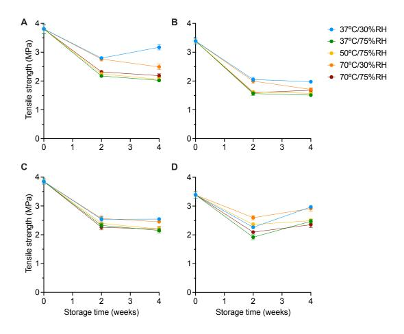
Figure E.3: The change in tensile strength for MCC/DCPA-based tablets with (A) CCS, (B) XPVP, (C) L-HPC and (D) SSG after storage under accelerated storage conditions for 2 and 4 weeks. Mean  $\pm$  standard deviation, n = 10.
