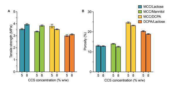
Figure 4.10: The (A) tensile strength and (B) porosity of tablets containing 5% and 8% w/w CCS, respectively.
