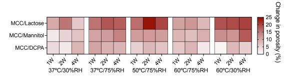
Figure 6.4: The mean relative change in porosity for tablets containing griseofulvin after storage under accelerated temperature and humidity conditions.
