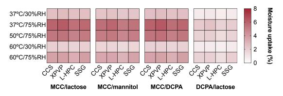
Figure 5.1: The theoretical moisture uptake for each formulation (%), based on the individual moisture sorption of each excipient.
