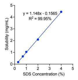
Figure 3.2: The solubility of griseofulvin in varying concentrations of SDS solution.
