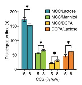
Figure 4.11: Disintegration times of batches prepared with 5% and 8% w/w CCS (n = 6; mean  $\pm$  standard deviation; \*p < 0.05)
