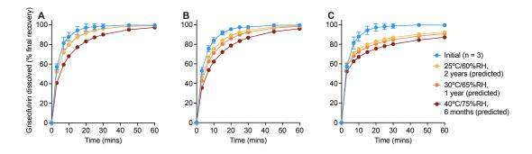
Figure 6.11: The predicted dissolution profiles for (A) MCC/lactose, (B) MCC/mannitol, and (C) MCC/DCPA tablets containing griseofulvin after storage under ICH long-term ( $25^{\circ}C/60\%$ RH), intermediate ( $30^{\circ}C/65\%$ RH), and accelerated ( $40^{\circ}C/75\%$ RH) storage conditions.
