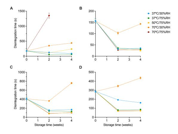
Figure E.13: The change in disintegration time for MCC/lactose-based tablets with (A) CCS, (B) XPVP, (C) L-HPC and (D) SSG after storage under accelerated storage conditions for 2 and 4 weeks. Mean  $\pm$  standard deviation, n = 6.
