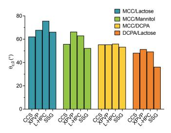
Figure 4.8: The initial contact angle of each formulation (n = 2)
