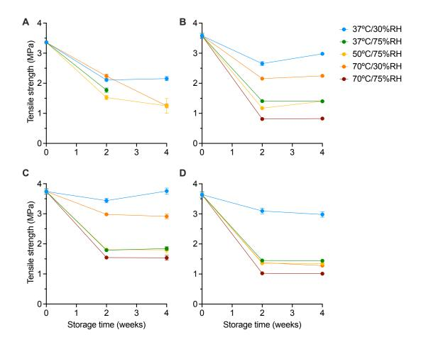
Figure E.2: The change in tensile strength for MCC/mannitol-based tablets with (A) CCS, (B) XPVP, (C) L-HPC and (D) SSG after storage under accelerated storage conditions for 2 and 4 weeks. Mean  $\pm$  standard deviation, n = 10.
