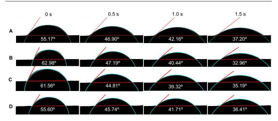
Figure 4.6: Examples of the contact angle measurements for MCC/mannitol-based tablets containing (A) CCS, (B) XPVP, (C) L-HPC and (D) SSG
