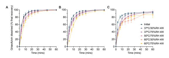
Figure 6.8: Dissolution profiles of (A) MCC/lactose-, (B) MCC/mannitol-, and (C) MCC/DCPA-based tablets containing griseofulvin before and after 4 weeks of storage under accelerated temperature and humidity conditions (mean  $\pm$  standard deviation, n =3 with the exception of the 60°C/30%RH and 60°C/75%RH condition for MCC/DCPA for which n=6).
