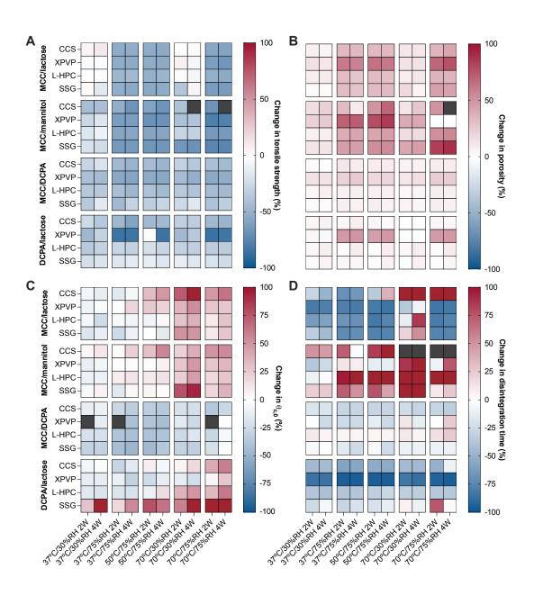
Figure 5.2: The change in (A) tensile strength, (B) porosity, (C)  $\theta_{c,0}$ , and (D) disintegration time for all batches after storage under accelerated conditions. Grey data points represent points where no data is available.
