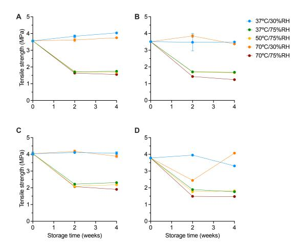
Figure E.1: The change in tensile strength for MCC/lactose-based tablets with (A) CCS, (B) XPVP, (C) L-HPC and (D) SSG after storage under accelerated storage conditions for 2 and 4 weeks. Mean  $\pm$  standard deviation, n = 10.
