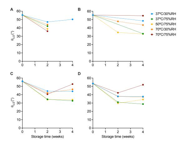
Figure E.11: The change in initial contact angle  $(\theta_{c,0})$  for MCC/DCPA-based tablets with (A) CCS, (B) XPVP, (C) L-HPC and (D) SSG after storage under accelerated storage conditions for 2 and 4 weeks. Mean, n = 2.
