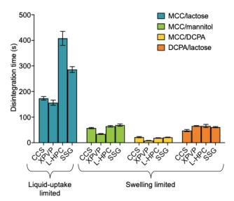
Figure A.1: Disintegration time (s) of each filler and disintegrant combination (showing mean and standard deviation).
