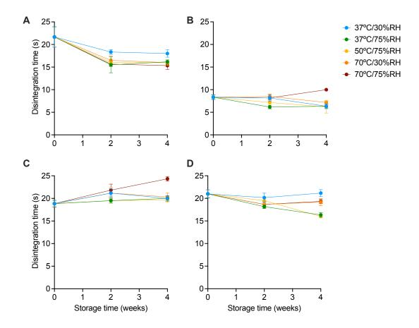
Figure E.15: The change in disintegration time for MCC/DCPA-based tablets with (A) CCS, (B) XPVP, (C) L-HPC and (D) SSG after storage under accelerated storage conditions for 2 and 4 weeks. Mean  $\pm$  standard deviation, n = 6.
