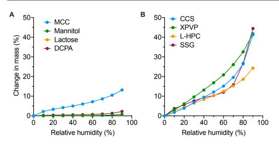
Figure 4.1: Moisture sorption isotherms of (A) fillers and (B) disintegrants
