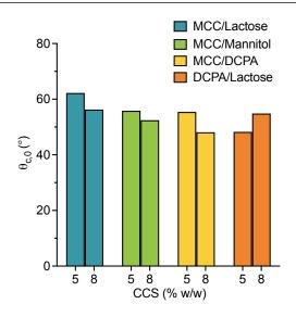
Figure 4.12: The initial contact angle,  $\theta_{c,0}$ , of tablets containing 5 and 8% w/w CCS (n = 2 and n = 4, for 5 and 8% w/w CCS, respectively).
