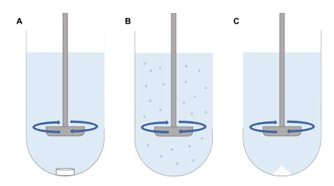
Figure 1.3: The USP II (paddle) apparatus (A) at the beginning of a dissolution test, (B) with dissolution in progress and the particles dispersed throughout the dissolution media as it stirs, and (C) with powder coning at the base of the vessel.
