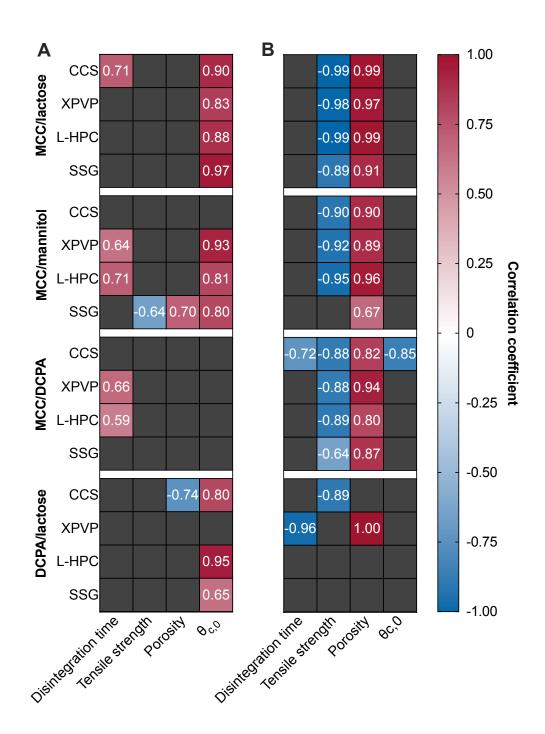
Figure 5.3: Pearson correlation coefficient between (A) storage temperature and (B) storage humidity with physical tablet properties. Only significant correlations (p < 0.05) are shown.
