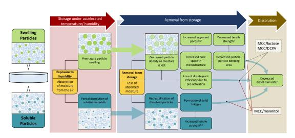
Figure 6.14: A summary of the potential mechanisms of physical change during the storage of tablets under accelerated conditions, including the expected effects on the physical tablet properties.
