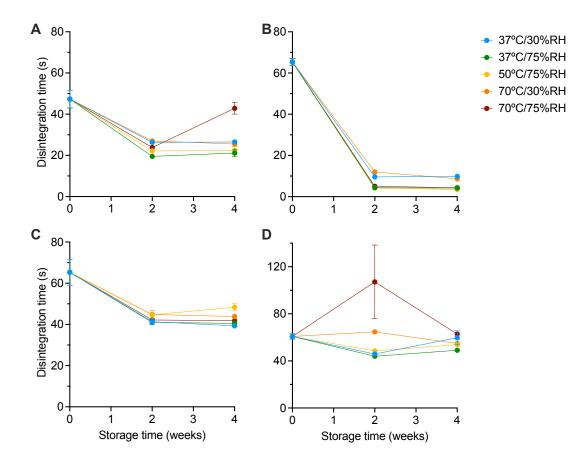
Figure E.16: The change in disintegration time for DCPA/lactose-based tablets with (A) CCS, (B) XPVP, (C) L-HPC and (D) SSG after storage under accelerated storage conditions for 2 and 4 weeks. Mean  $\pm$  standard deviation, n = 6.
