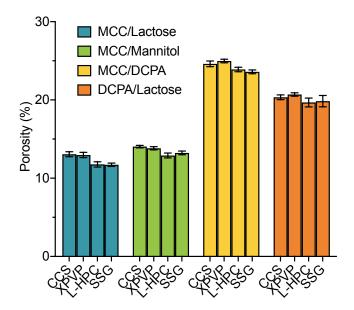
Figure 4.4: The porosity of each formulation  $(n = 10, \text{mean} \pm \text{standard deviation})$
