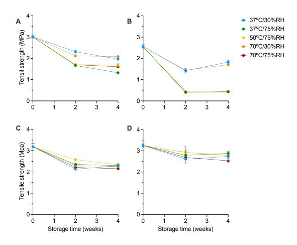
Figure E.4: The change in tensile strength for DCPA/lactose-based tablets with (A) CCS, (B) XPVP, (C) L-HPC and (D) SSG after storage under accelerated storage conditions for 2 and 4 weeks. Mean  $\pm$  standard deviation, n = 10.
