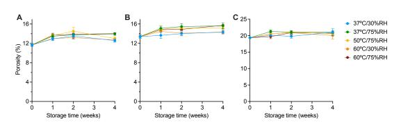
Figure 6.3: The porosity of (A) MCC/lactose-, (B) MCC/mannitol-, and (C) MCC/DCPA-based tablets containing griseofulvin before and after storage under accelerated temperature and humidity conditions (mean  $\pm$  standard deviation, n = 210 at 0 weeks, and n = 14 at subsequent timepoints).
