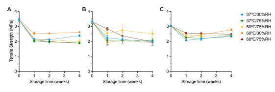
Figure 6.2: The tensile strength of (A) MCC/lactose-, (B)MCC/mannitol-, and (C) MCC/DCPA-based tablets containing griseofulvin before and after storage under accelerated temperature and humidity conditions (mean  $\pm$  standard deviation, n = 4).
