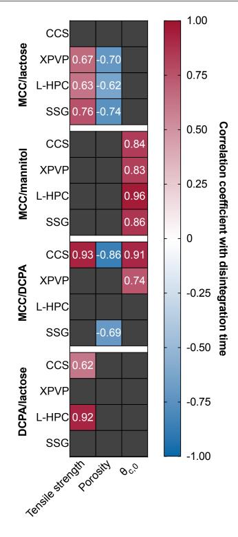
Figure 5.4: Pearson correlation coefficient between the disintegration time and the tensile strength, porosity and initial contact angle of all tablet during storage. Only significant correlations (p < 0.05) are shown.
