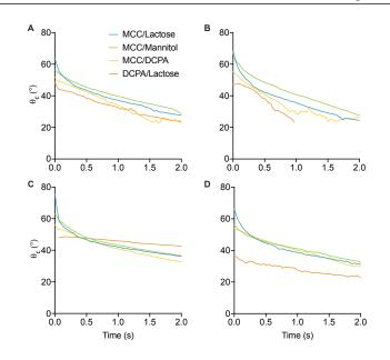
Figure 4.7: Contact angle profiles of tablets containing (A) CCS, (B) XPVP, (C) L-HPC and (D) SSG (n = 2)
