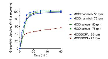
Figure 6.7: The dissolution profiles of griseofulvin from tablets composed of MCC/mannitol, MCC/lactose, and MCC/DCPA with paddle speeds of 50 and 75 rpm, shown as a percentage of the final release of griseofulvin after a 30 min infinity spin at 200 rpm.
