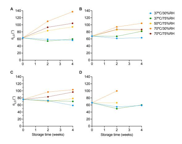
Figure E.9: The change in initial contact angle  $(\theta_{c,0})$  for MCC/lactose-based tablets with (A) CCS, (B) XPVP, (C) L-HPC and (D) SSG after storage under accelerated storage conditions for 2 and 4 weeks. Mean, n = 2.
