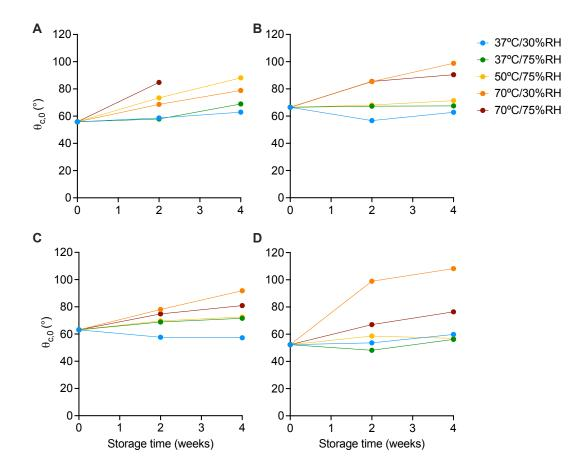
Figure E.10: The change in initial contact angle  $(\theta_{c,0})$  for MCC/mannitol-based tablets with (A) CCS, (B) XPVP, (C) L-HPC and (D) SSG after storage under accelerated storage conditions for 2 and 4 weeks. Mean, n = 2.
