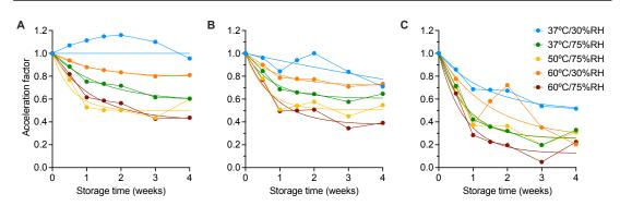
Figure 6.9: The acceleration factors of (A) MCC/lactose, (B) MCC/mannitol, and (C) MCC/DCPA, using experimental values (0, 1, 2, and 4 weeks) and values imputed by spline interpolation (0.5, 1.5, and 3 weeks), including the fit of a first-order exponential decay curve for each condition.
