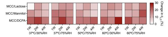
Figure 6.5: The relative change in  $\theta_{c,0}$  after 1, 2 and 4 weeks storage at accelerated temperature and humidity conditions (mean of n = 4).
