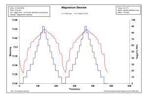
Figure D.2: Settling plot from the dynamic vapour sorption measurement of magnesium stearate.
