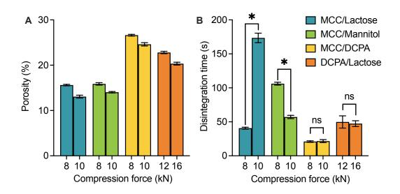
Figure 4.9: The (A) porosity and (B) disintegration time of tablets compressed at 8 and 10 kN (MCC/lactose, MCC/mannitol and MCC/DCPA) or 12 and 16 kN (DCPA/lactose). n = (A) 10 or (B) 6; mean  $\pm$  standard deviation; \*p < 0.05; ns: not significant.
