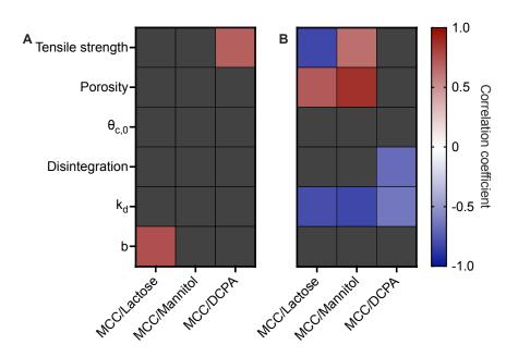
Figure 6.13: Pearson correlation coefficients between (A) temperature and (B) humidity with the change in physical tablet properties during storage. Only significant correlations (p < 0.05) are shown.
