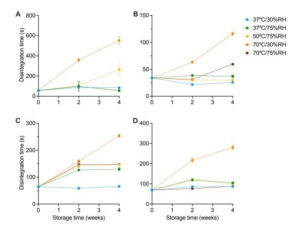
Figure E.14: The change in disintegration time for MCC/mannitol-based tablets with (A) CCS, (B) XPVP, (C) L-HPC and (D) SSG after storage under accelerated storage conditions for 2 and 4 weeks. Mean  $\pm$  standard deviation, n = 6.
