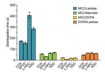
Figure 4.5: The disintegration time of each formulation  $(n = 6, \text{mean} \pm \text{standard} \text{deviation})$
