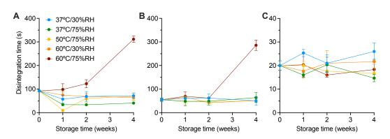
Figure 6.6: The disintegration time of griseofulvin tablets containing (A) MCC/lactose, (B) MCC/mannitol, and (C) MCC/DCPA after storage under accelerated conditions (mean  $\pm$  standard deviation, n = 3).
