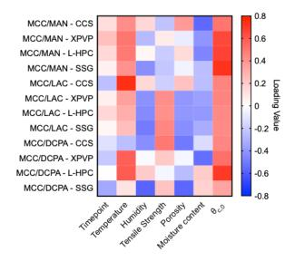
Figure A.2: Loading values from the PLS analysis of MCC/mannitol, MCC/lactose and MCC/DCPA formulations with each disintegrant.  $\theta_{c,0}$  is the initial contact angle.
