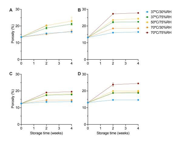
Figure E.6: The change in porosity for MCC/mannitol-based tablets with (A) CCS, (B) XPVP, (C) L-HPC and (D) SSG after storage under accelerated storage conditions for 2 and 4 weeks. Mean  $\pm$  standard deviation, n = 100 (0 weeks) and n = 10 (2 and 4 weeks).
