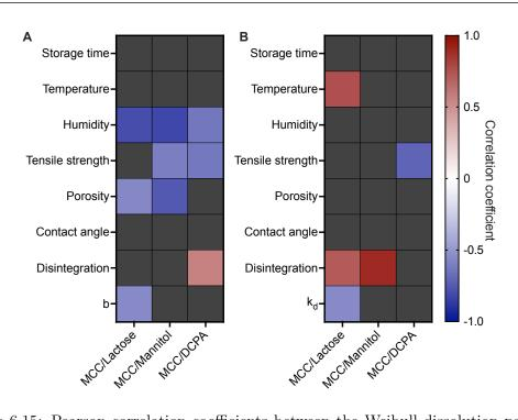
Figure 6.15: Pearson correlation coefficients between the Weibull dissolution parameters, (A)  $k_s$  and (B) b, with the change in physical tablet properties during storage. Only significant correlations (p < 0.05) are shown.
