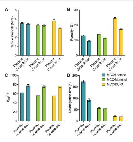
Figure 6.12: The (A) tensile strength, (B) porosity, (C) initial contact angle ( $\theta_{c,0}$ ) and (D) disintegration time of placebo tablets (see Chapter 4) and griseofulvin tablets prior to storage (mean  $\pm$  standard deviation, except for (C) where n = 2 for placebo tablets and so no standard deviation is shown).
