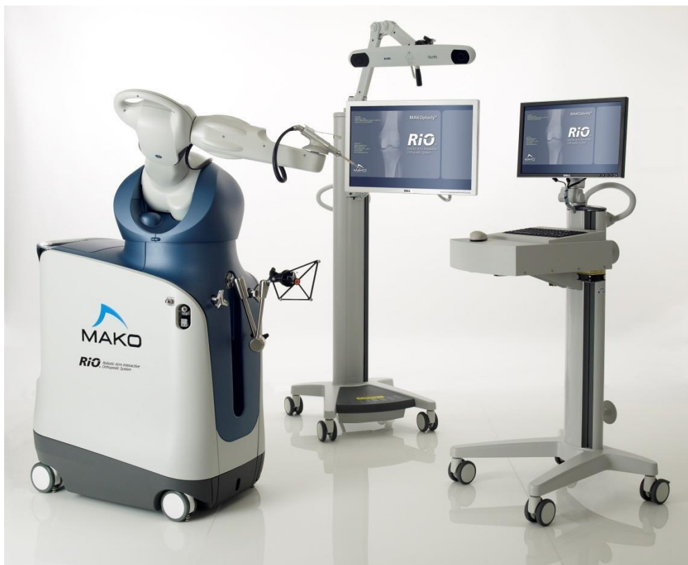
Figure1.6: the components of the MAKO RIO system employed in partial knee MAKOPlasty, showing (from left to right) the robotic arm with burr, the stereoscopic infrared optical tracking system and the control panel.
