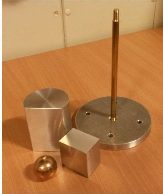
Figure 4.1: The three test pieces used: a sphere, cuboid and flattened off cylinder. Also shown is the mount, to which each was attached to allow full access.
