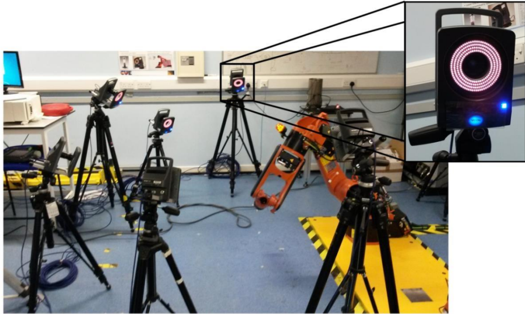
Figure 3.11: The camera setup relative to the robot position, with all cameras on one side of the robot, due to spatial constrictions in the robot cell. Also detailed is the face of one of the cameras, showing the LED strobe ring and the lens in the centre.
