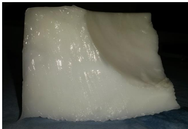
Figure 8.9: A quarter of the tissue mimic material, cut from the container using a scalpel, displaying an isotropic dispersion of powder.
