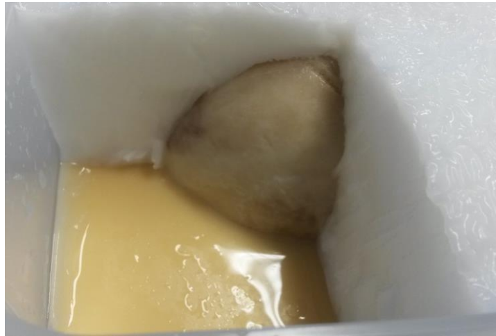
Figure 8.10: The partially exposed sample after removal of a quarter of the tissue mimic material, showing small gaps between the osseous tissue and the mimic.
