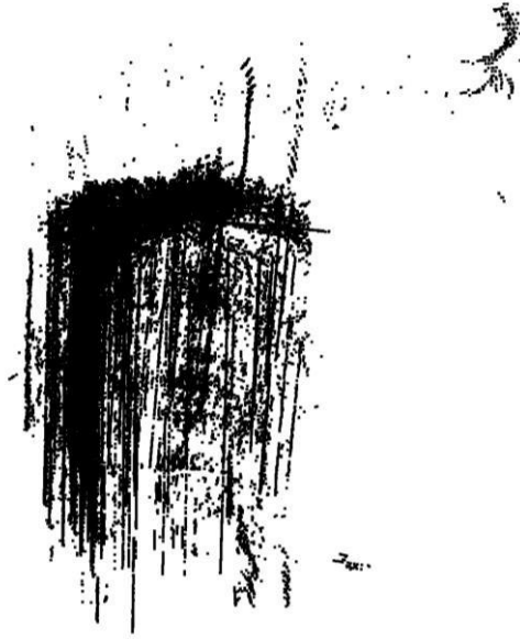
Figure 4.31: The TFM-derived point cloud resulting from the hemispherical scan. The threshold limit employed was -5dB. The increase in threshold has resulted in lower side lobe extraction, but has also resulted in true surface extraction also.
