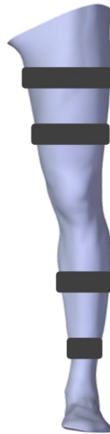
Figure 9.9: Possible position of immobilisation straps that would ensure no movement of the joint during ultrasonic bone surface capture.
