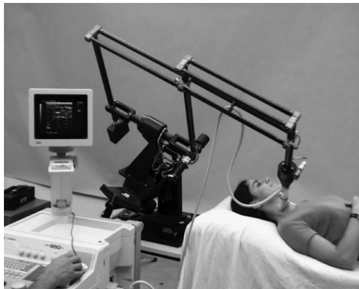
Figure 1.8: The system described by (Abolmaesumi et al., 2002) for imaging of the carotid artery ©[2002] IEEE. The probe maintains good contact with the skin using movement of the manipulation system, which is controlled by an external expert.
