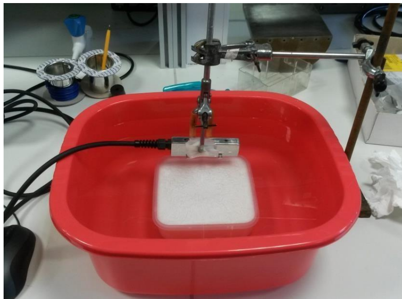
Figure 8.2: The apparatus used to retrieve FMC data from the condylar surface whilst situated in soft tissue mimicking material.
