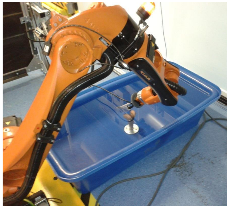
Figure 5.4: The physical setup of the experiment, showing the robot with probe attached, manoeuvring around the composite bone. The bone was completely submerged in tap water, as was the face of the probe.
