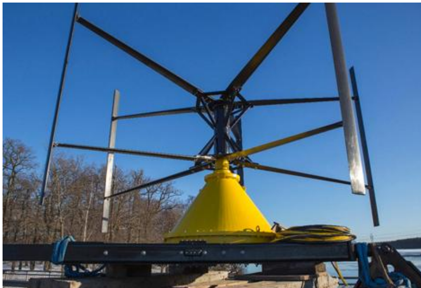
(b) Uppsala University Söderfors 30 kW turbine as deployed in the Dalälven river, Sweden (from von Schultz, 2013)
