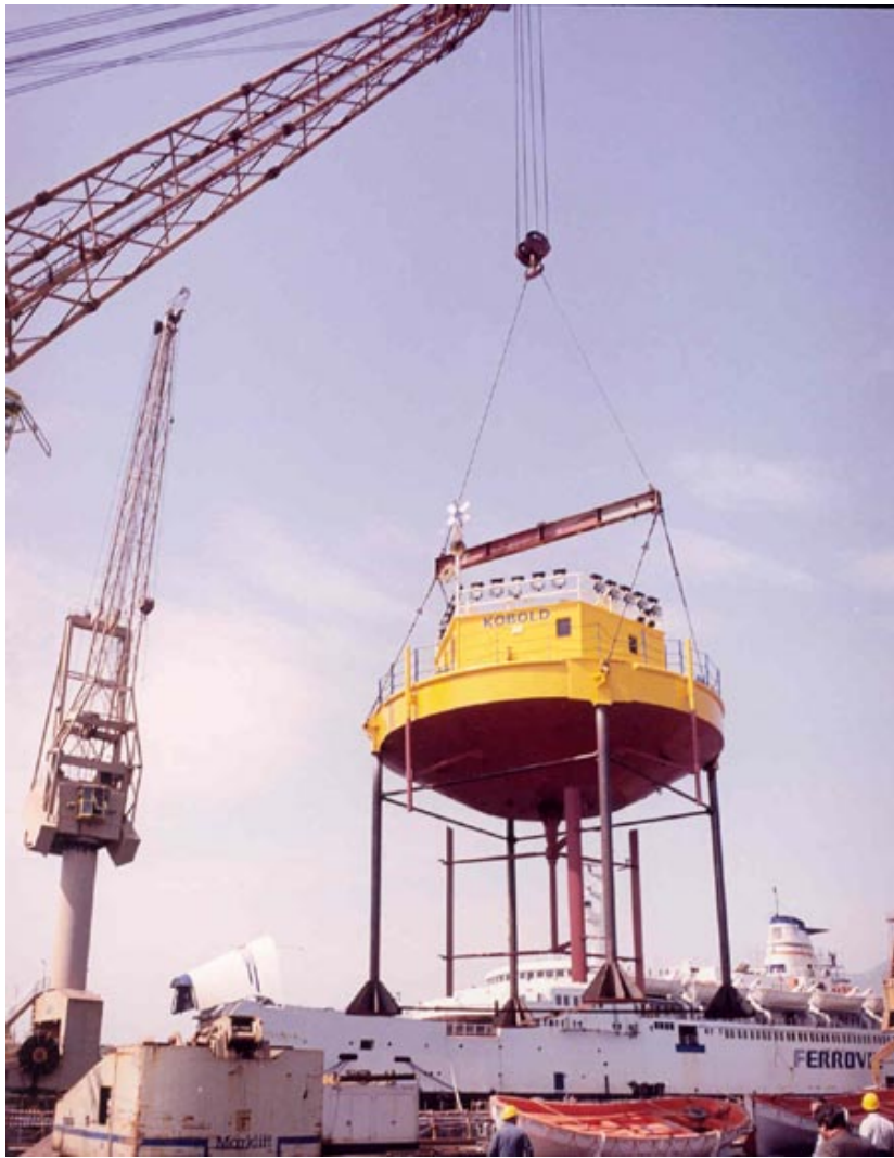
(a) Kobold ENERMAR 160 kW turbine as deployed in the Straits of Messina, Italy (from Ponte di Archimede International S.p.A., 2012)
