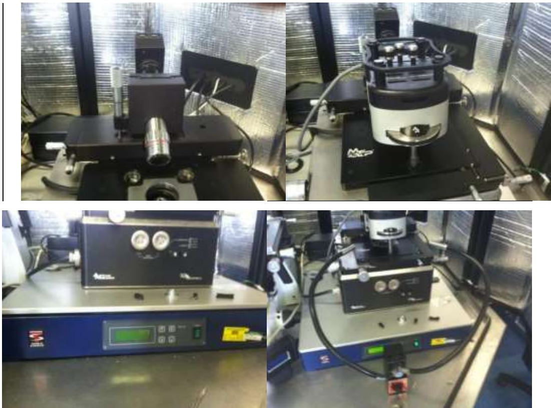
Figure 4: Asylum Research Nanoindenter system with vibration isolation table and external light source.
