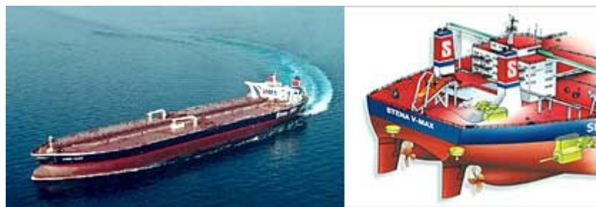
Figure 7.18: The double-rudder arrangement can improve the manoeuvrability of larger ships and reduce the chances of unwanted incidents, ( www.concordia-maritime.se )
