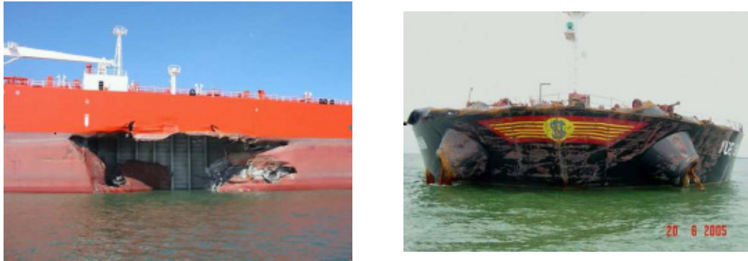
Figure 5.2: The highly localised character of collision is demonstrated in this picture. The imprint of the striking vessel (right) is clearly seen, (BMT, 2005)
