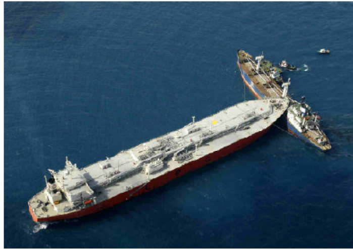
Figure 5.1: The bow of the significantly larger striking ship is driven substantially into the side of the struck vessel ( http://www.cargolaw.com/2003nightmare_t-bone.html )
