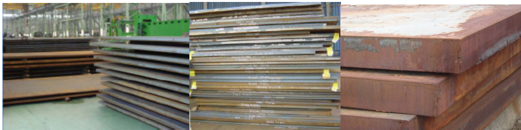
Figure 3.10. Monopile manufacturing. Storage of steel plates [82]
