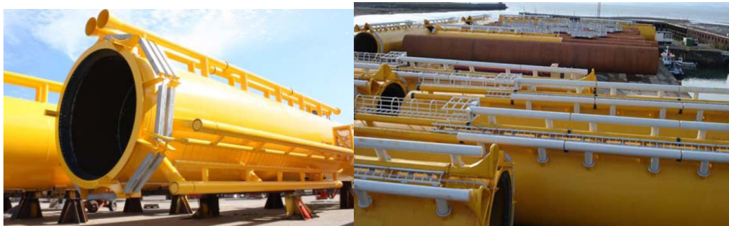
Figure 3.23. Monopile manufacturing. Coating [82]
