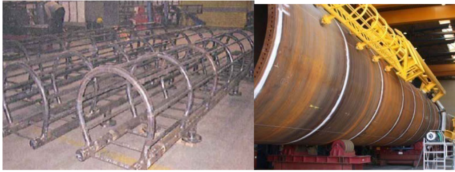
Figure 3.22. Monopile manufacturing. Secondary steel assembly [82]
