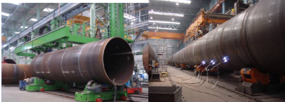
Figure 3.20. Monopile manufacturing. Outside circular welding [82]
