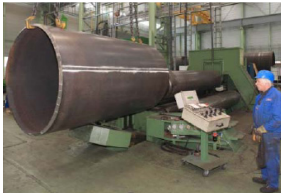
Figure 3.16. Monopile manufacturing. Calibration [82]
