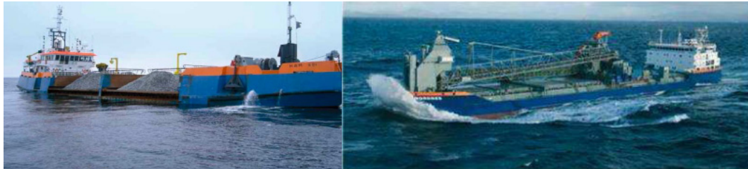
Figure 3.29. Side stone dumping vessel (on the left) and flexible fall pipe vessel (on the right) [89]
