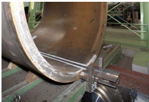
Figure 3.14. Monopile manufacturing. Milling of the longitudinal union [82]
