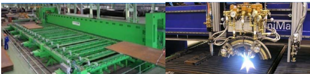
Figure 3.11. Monopile manufacturing. Milling and cutting [82]
