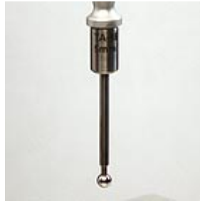
Figure 2- 20 5mm stainless steel pin head probe used for texture analysis measurements (Technologies, 1998-2011).
