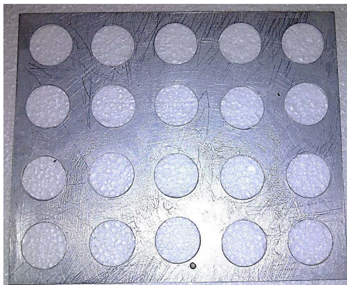
Figure 2- 2 Metal curing plate for UV synthesis of thiol-ene polymers. Aluminium foil coated onto one side using vacuum grease as fixative before wells (2 cm diameter) filled with reaction mixture and curing taking place.
