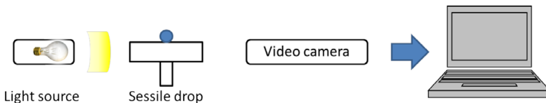
Figure 2- 3 Basic components of a contact angle goniometer.
