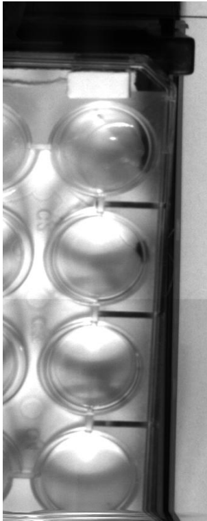
Figure 4- 22 Raw image of polymer disc coated in bacteria (well 1, top), positive bacterial polystyrene control (well 2, second), negative polystyrene control (well 3, third) and finally an empty well (well 4, bottom).
