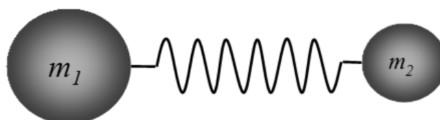
Figure 2.1: Schematic depicting a simple diatomic molecule as two masses ( m_1 and m_2 ) attached by a spring. 5
