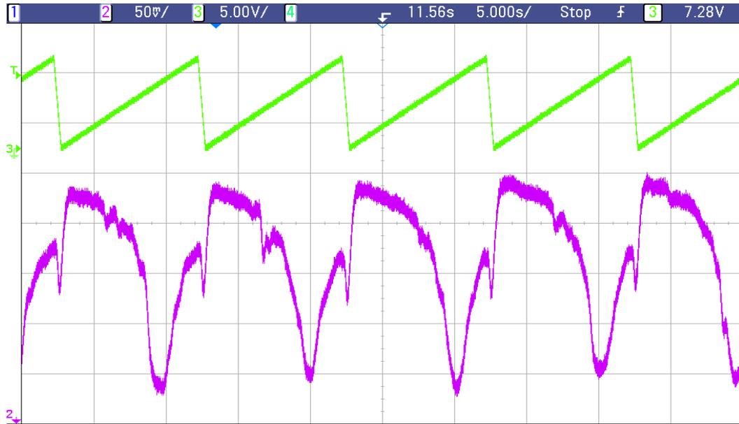
Figure 3.50: Gas detection along the line shape with 1f of LIA output
