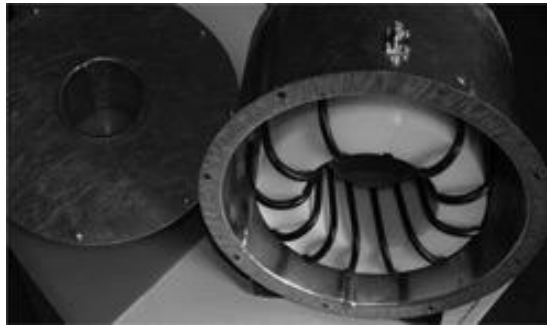
Figure 2.16: Rogowski coil placed in a metal enclosure [58].
