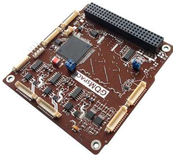
Figure 3.2: Nanomind On-Board Computer (OBC) from GomSpace.
