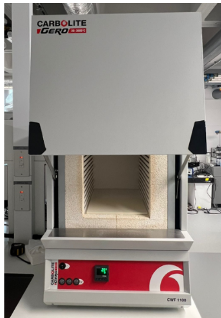
Figure 4.12: The Carbolite Furnace for annealing samples
