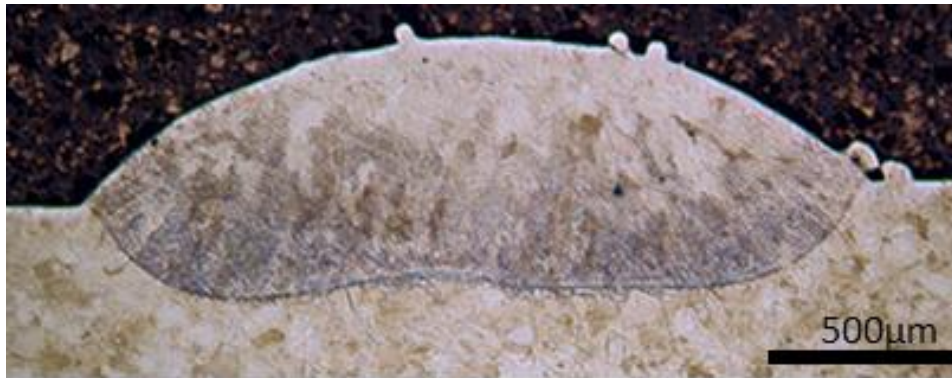
Figure 4.20 Fused partially melted powder with P=950W .
