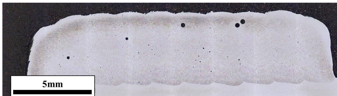
Figure 4.29 Cross section of high laser power ( P=950\text{W} ) full solid block made by stitching multiple optical micrographs together.
