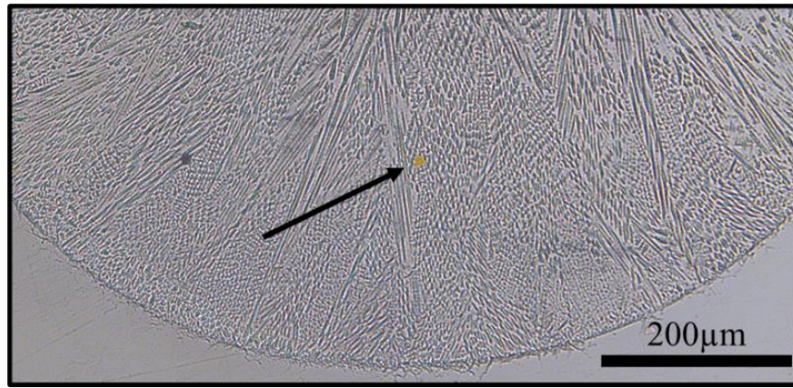
Figure 4.25 (a) Single track cross sections for 750W laser power showing the presence of primary carbide phases present at the liquid-solid interface.
