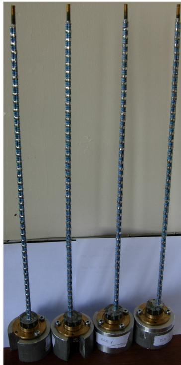
Fig. 7. 18 A photograph of the voltage dividers.
