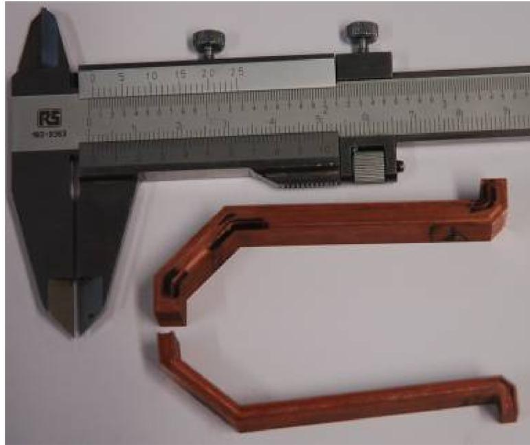
Fig. 3. 23 The waveguide bend.
