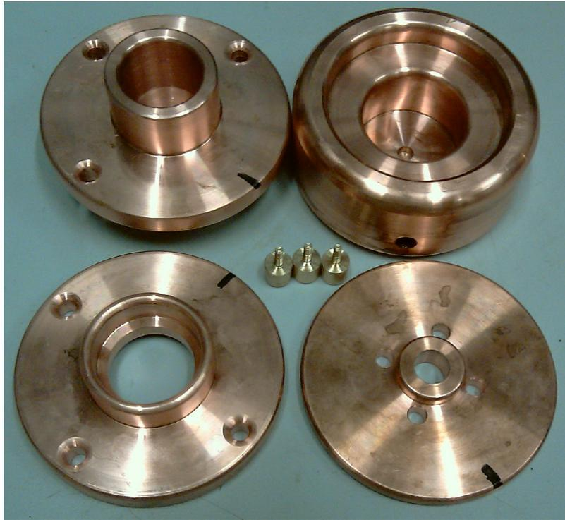
(b) The electrodes of the depressed collector;
