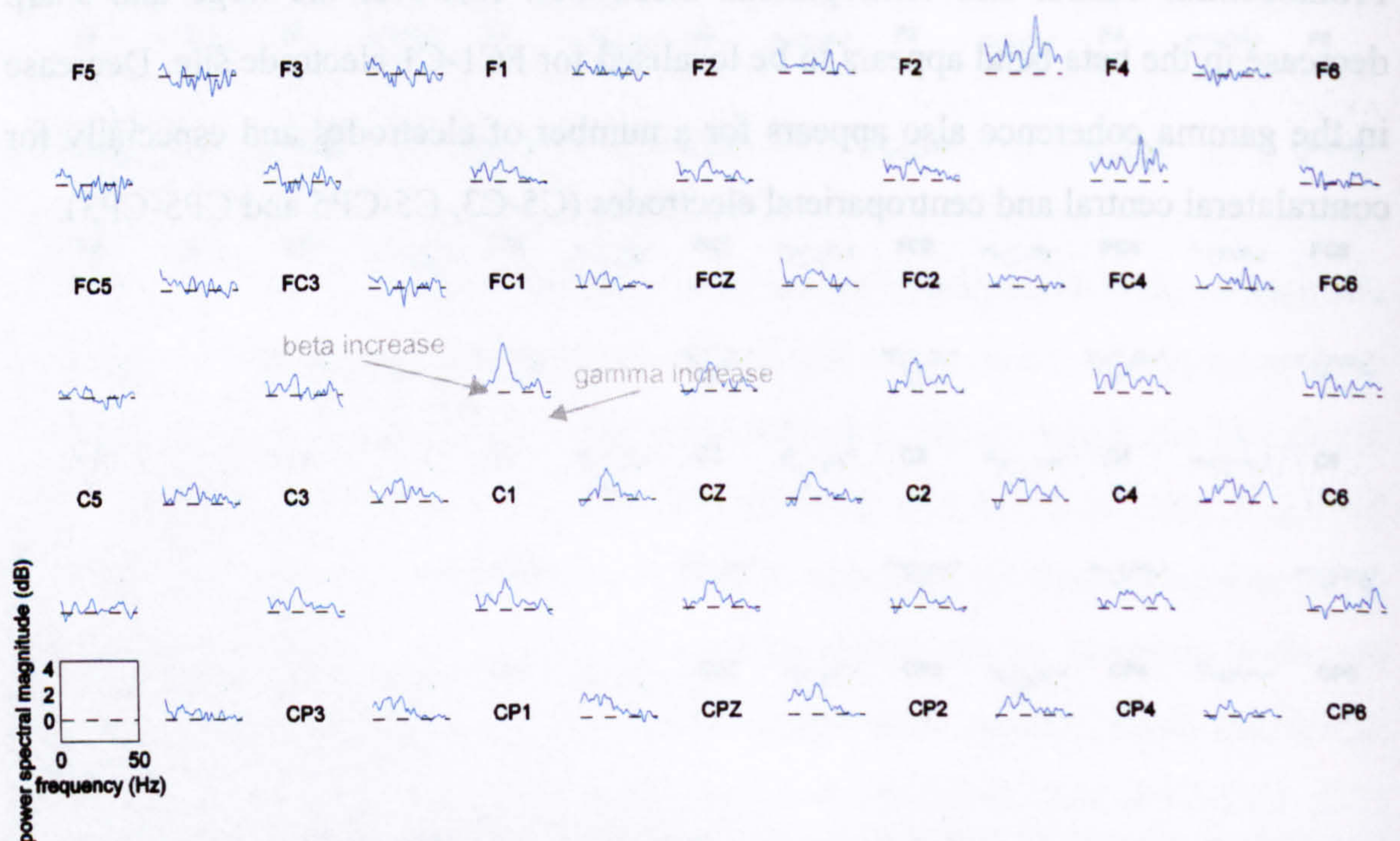
Fig. 5.27 EEG bipolar power spectral difference map between movement extension and posture extension, pooled power spectral maps. The labels represent the relative position of the electrodes over the head. The green vertical line indicates the magnitude of a 95% confidence interval for the spectral estimates.
