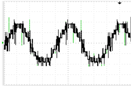
e) Line voltage Scale: (50ms/Div-x-axis, 100V/Div-y-axis)
