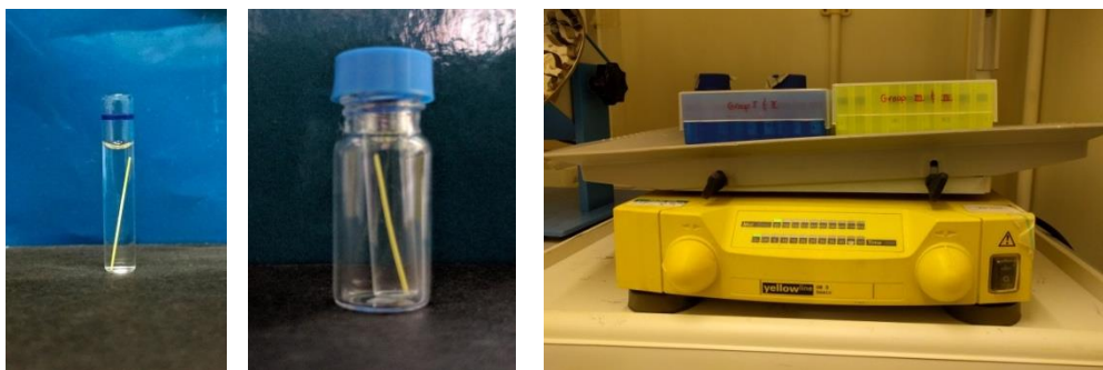
Figure 4.4: In vitro drug release setup showing the implants suspended in PBS in a glass insert. The inserts are placed in glass vials on batch shaker in a thermostatically controlled temperature room at 37°C
