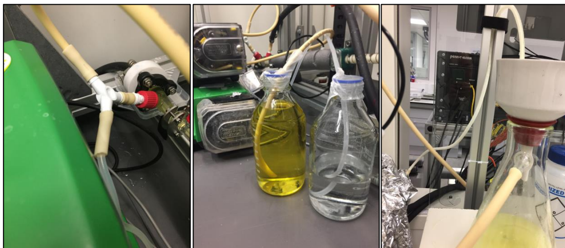
Figure 7.8 Y-piece to flow streams (left), stock solutions of individual streams ALA in IPA and NIC in water (centre) and filtration set up (right).
