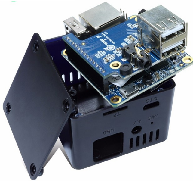
Figure 3.5: OrangePi Zero Plus2 with expansion board and cubic case. Image from [29]
