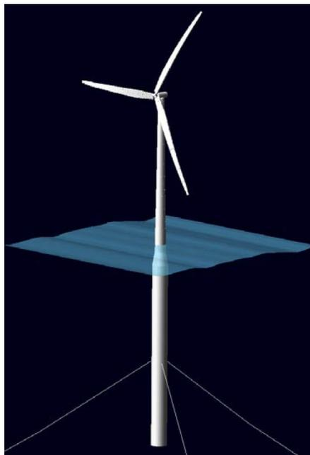
**Figure 3.4:** The OC3 phase IV spar-buoy FOWT system (Jonkman 2010).
