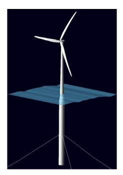
Figure 3.4: The OC3 phase IV spar-buoy FOWT system (Jonkman 2010).
