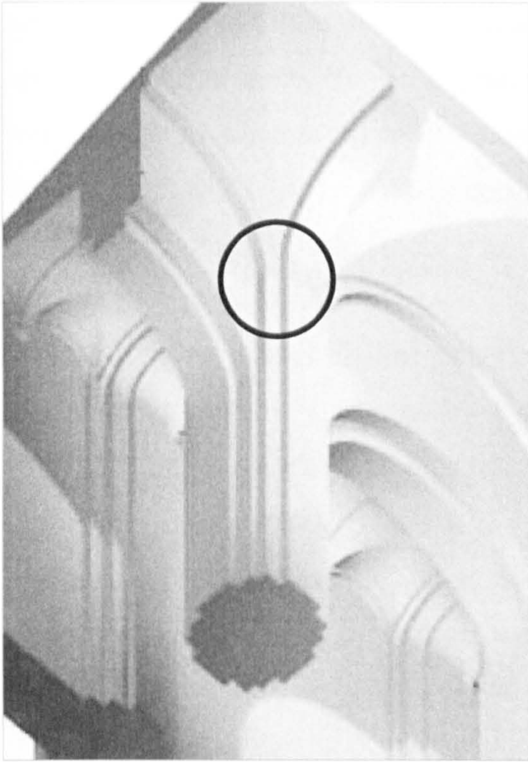
Fig 6.7 Groin vault rising between profiles of giant order
