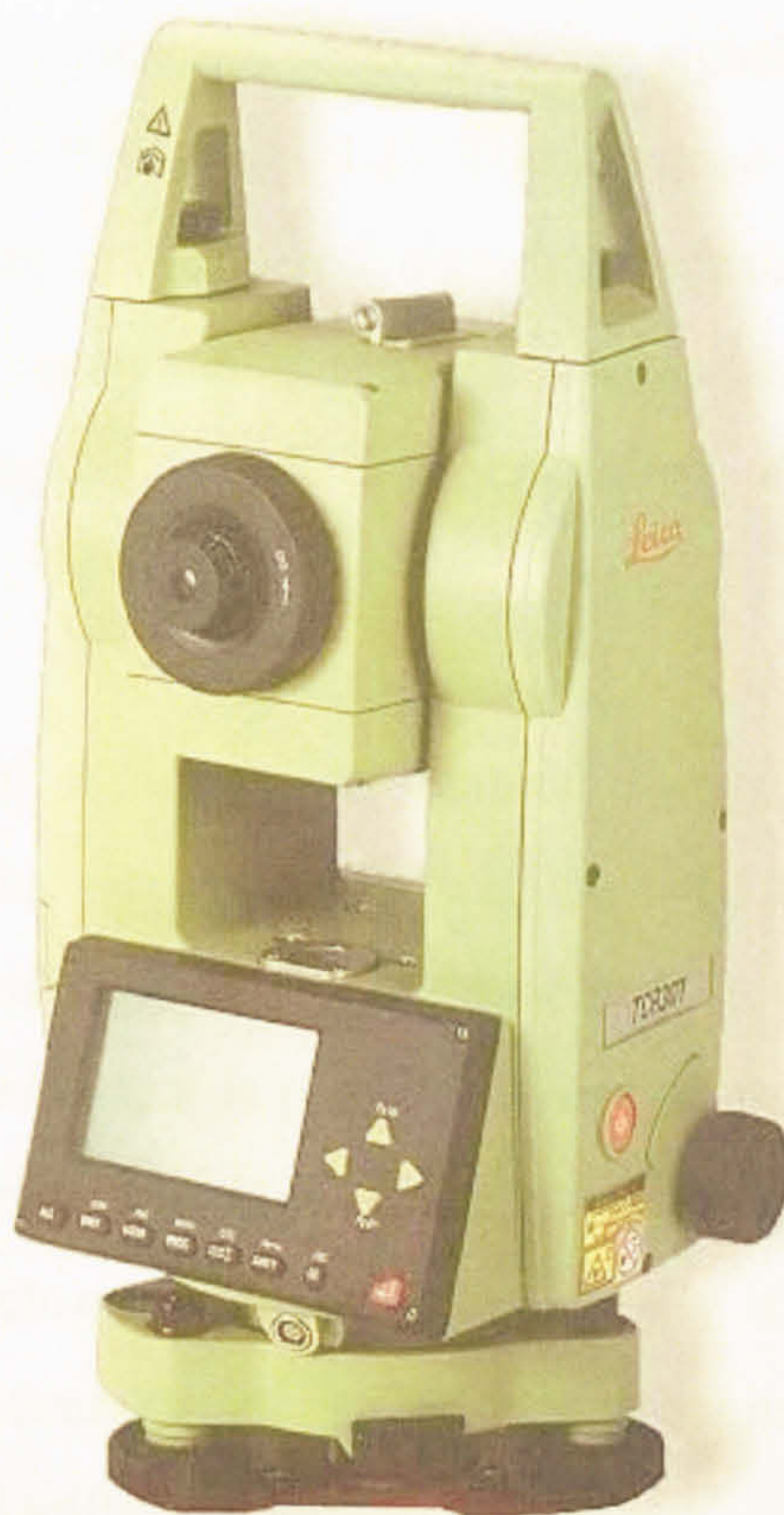
Fig. 4.2 A total station (from Leica Geosystems 2005)
