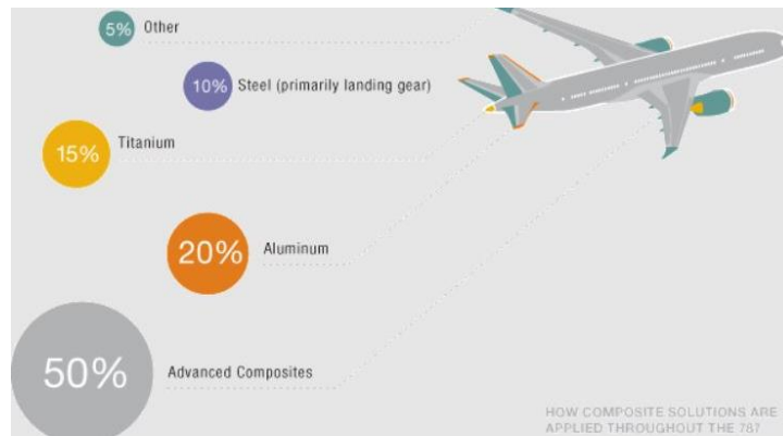
Figure 2.7. Material use as weight percentage in a Boeing 787 passenger jet [35].
