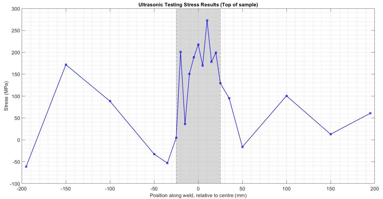
Figure 46: Mean PAURS RS distribution across the top surface of the welded S275 specimen.
