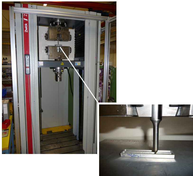
Fig. 15: Universal testing machine 'Zwick BX100/SN5A' with flaring test setup
