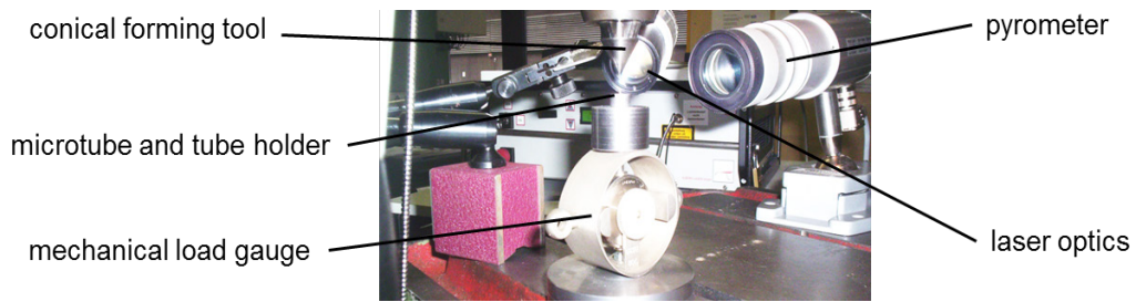
Fig. 19: Experimental setup (early laser-assisted trials)
