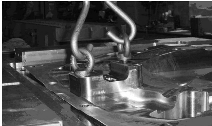
Fig. 69: Rapid interchange ability of separate inserts (Schuler)
