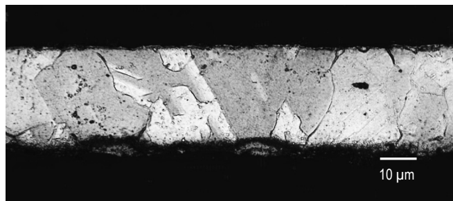
Fig. 97: Microstructure of the recrystallized AISI 304-r micro-tube
