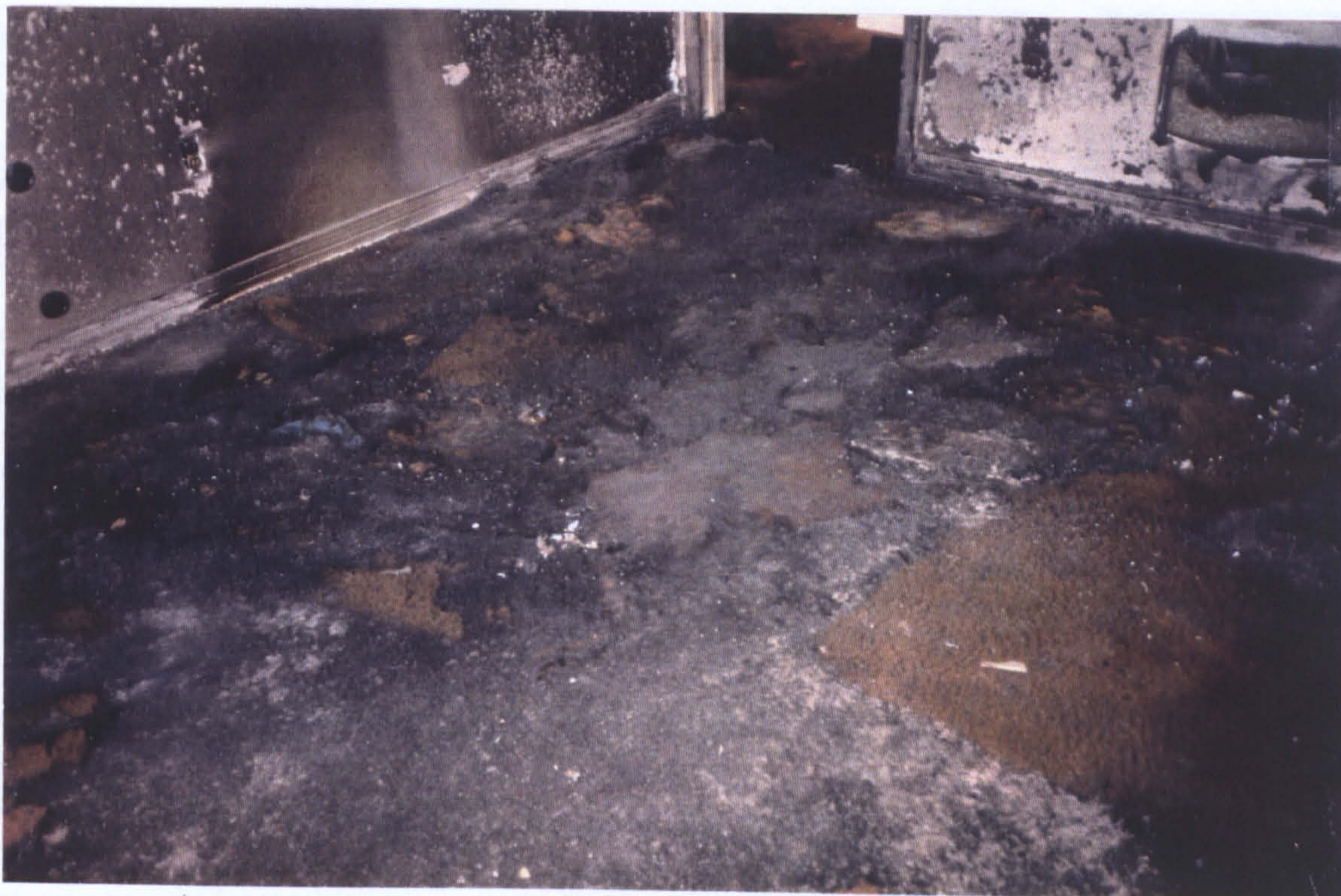
Fig. A3.10.4.14: A furnished, carpeted room (B1) similar to that used in previous tests was ignited with direct flame applied to the bed with no flammable liquid accelerants present. Fire proceeded to flashover at ~46min after ignition and was extinguished as flashover progressed. The charred areas of carpet in the centre of the room were the result of radiant heat from the ceiling layer and from adjacent items of clothing and furnishings. Large unburned areas were the result of protection offered by those other fuels.
