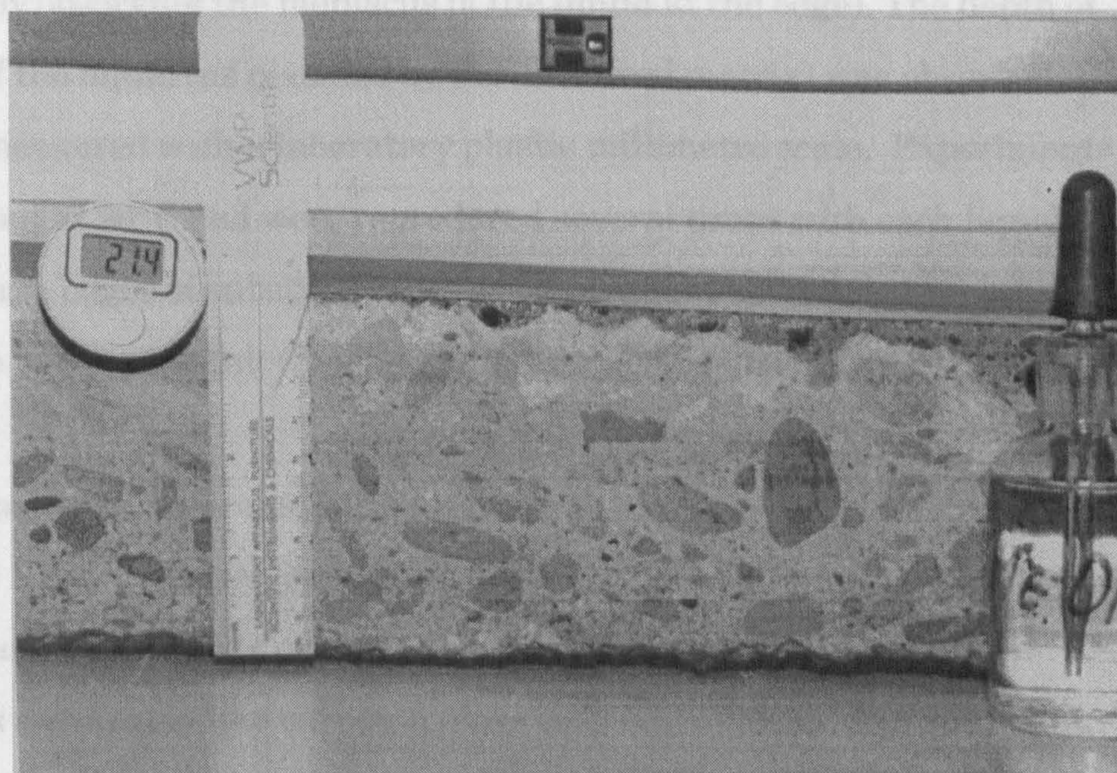
Fig. 2.1.2: Typical depth penetration – methanol on concrete.
