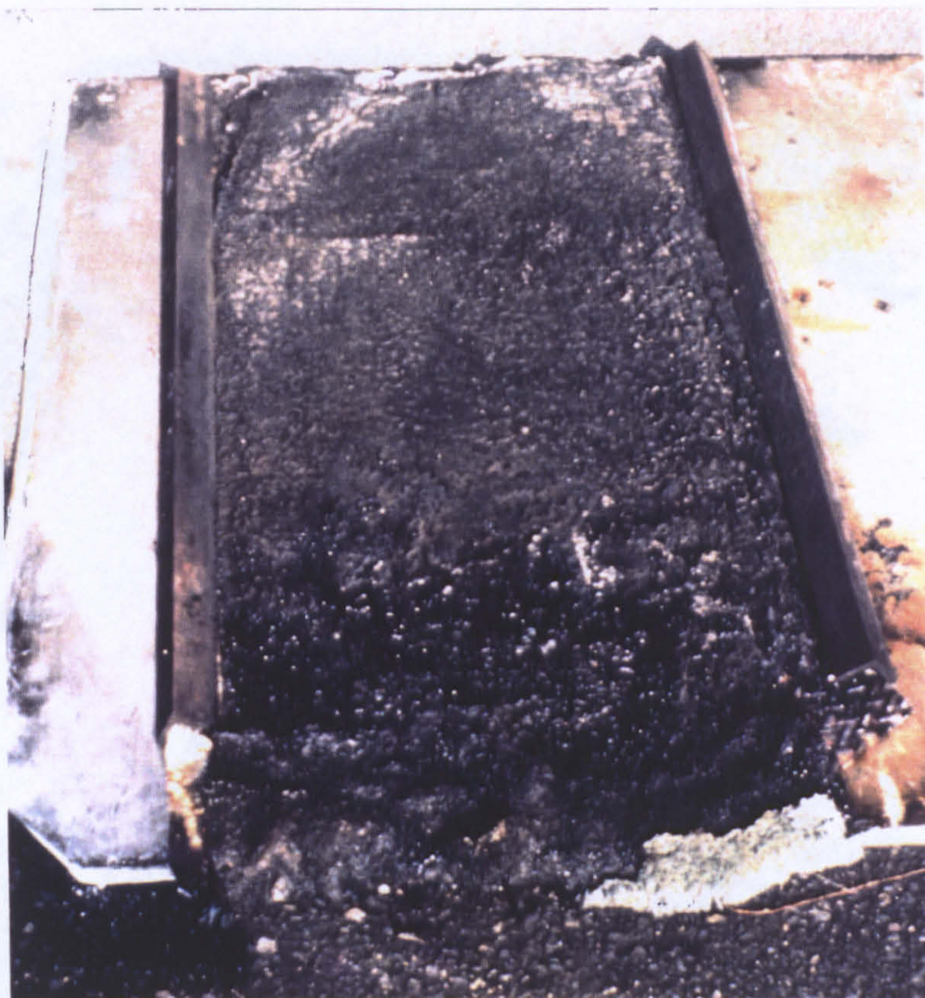
Fig. 3.10.4.4: Nylon plush (16mm pile) carpet after ignition with 1.9 litres of camping fuel (Test 10) in a normally-ventilated room. Pile and backing largely destroyed by 7min of fire, especially at the end facing the ventilation source (door).
