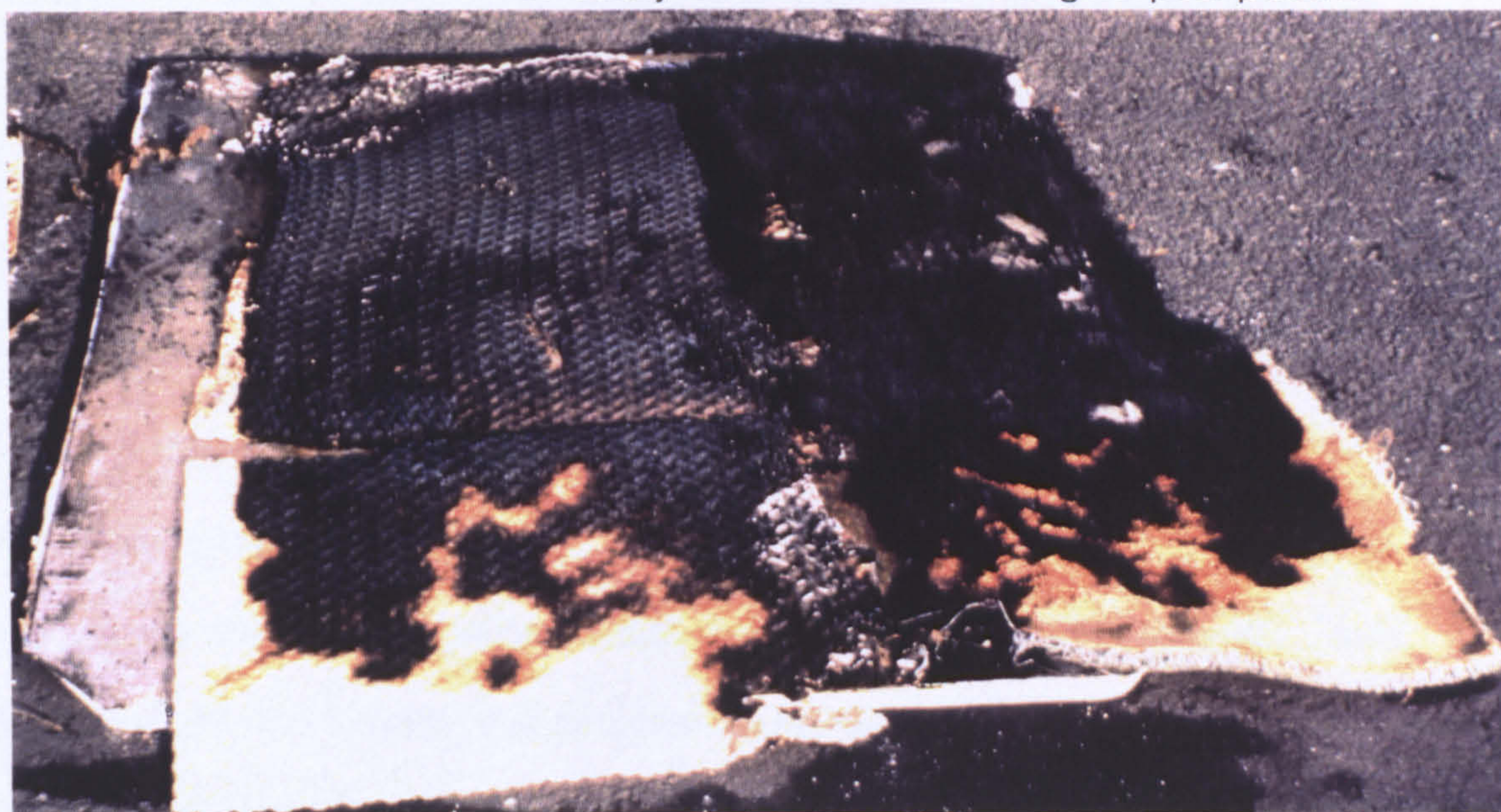
Fig. 3.10.4.7: Same carpet panel after reversal to reveal damage to rubber pad beneath. Most of damage to pad cannot be linked to shape of original pour pattern. Note more extensive damage to carpet due to longer burning time. The H-shaped pattern of penetrations (marked by white areas on carpet and corresponding localized deep damage to pad) are in the shape and location of the pour pattern.
