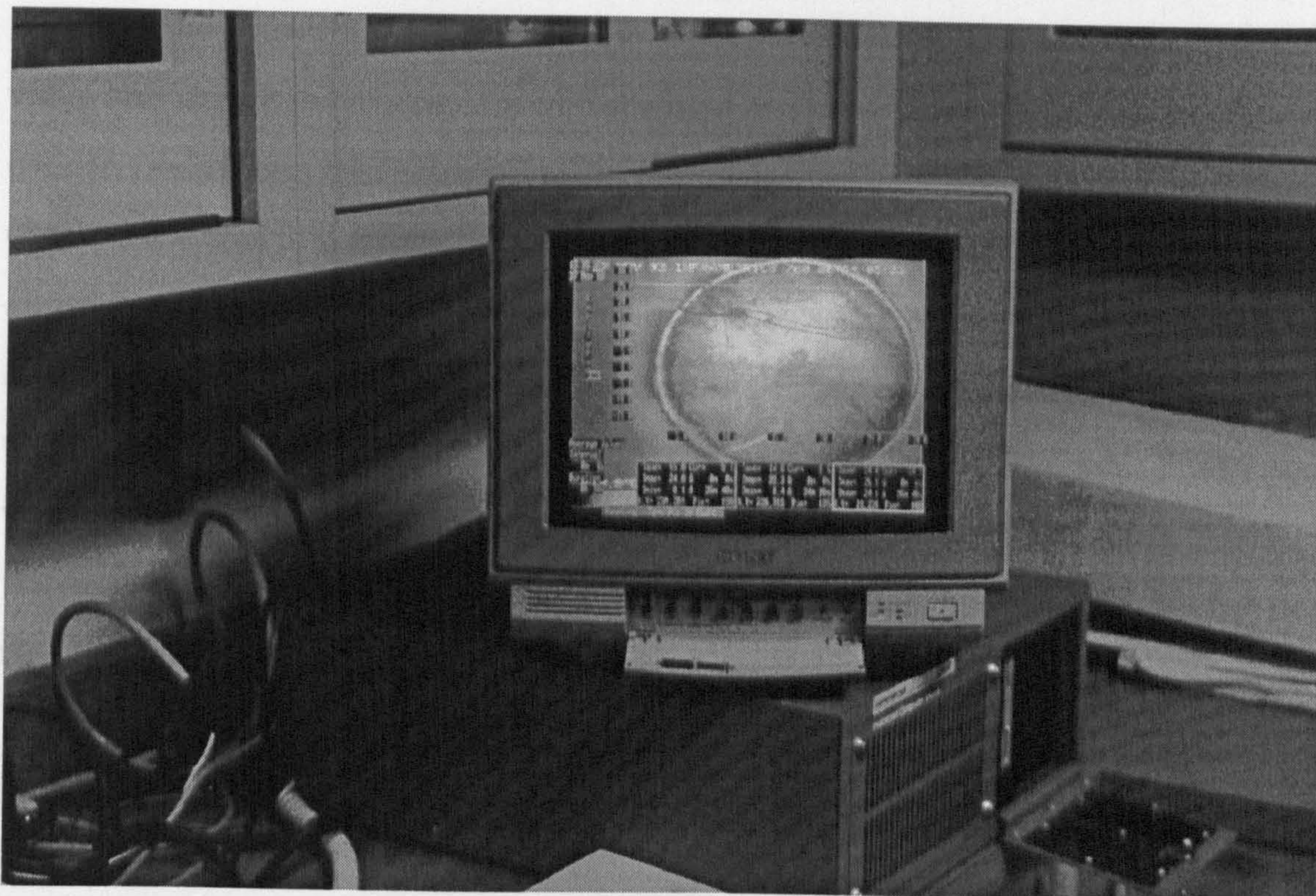
The calibration of the infrared thermal imaging system is dependent on Fig. 2.8.2.2: Video display of ThermaGram© Data System showing the thermal video (false-colour) image of the evaporating sample along with overlying traces recording the temperatures at three selected sampling points within the image. The image is of pentane on sand. Note the irregularities in the surface temperature.
