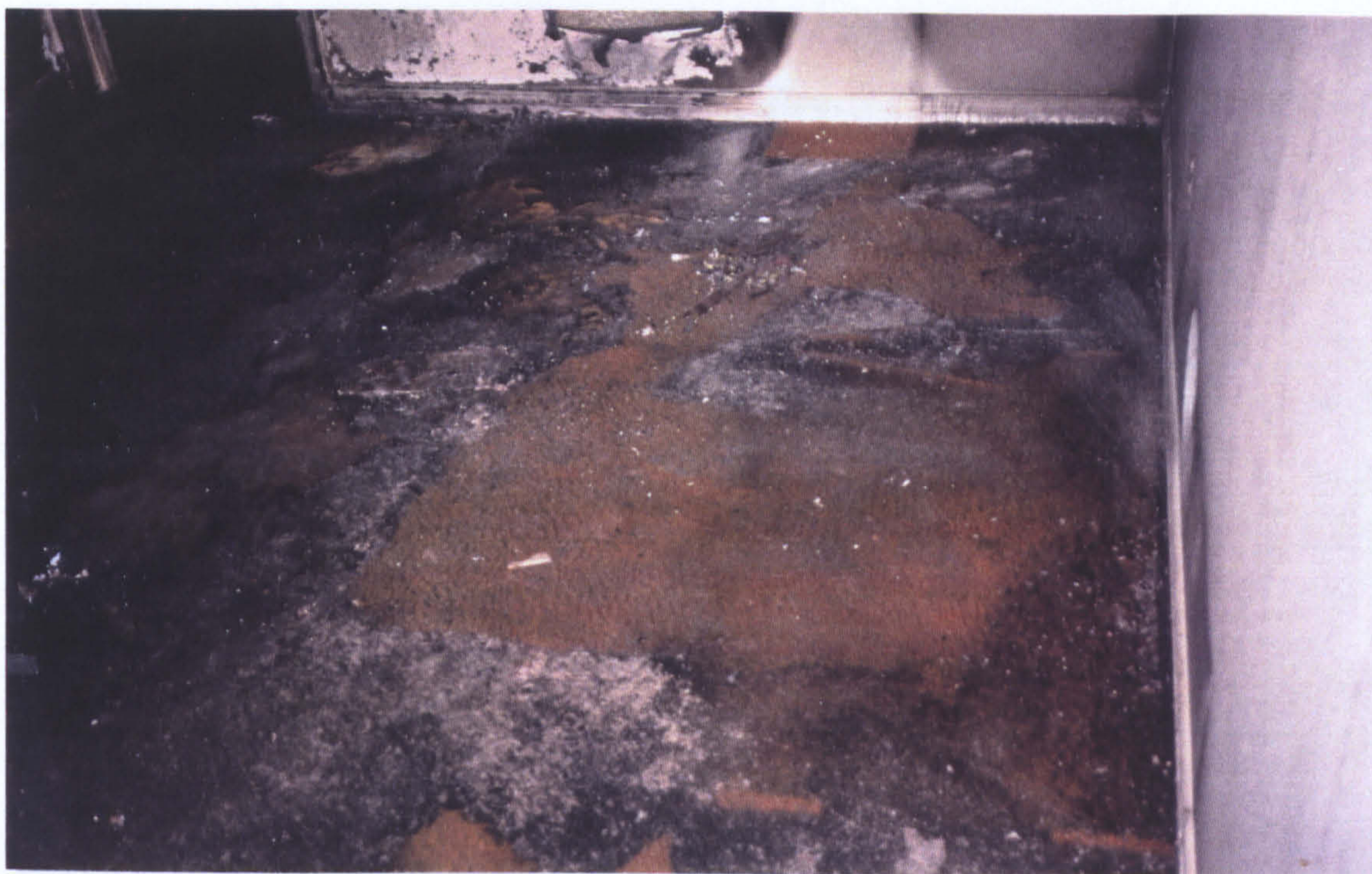
Fig. A3.10.4.12: Results of room test (B4) where ~3litres of camping fuel was poured in a random pattern across a furnished, carpeted room and ignited. The fire was extinguished less than 3min after ignition so the room was not allowed to proceed to flashover. Large areas of undamaged carpet are visible. The deep, localized damage is in the same area as the primary pour of fuel but is larger than the pool that could be produced from the quantity of fuel actually poured.
