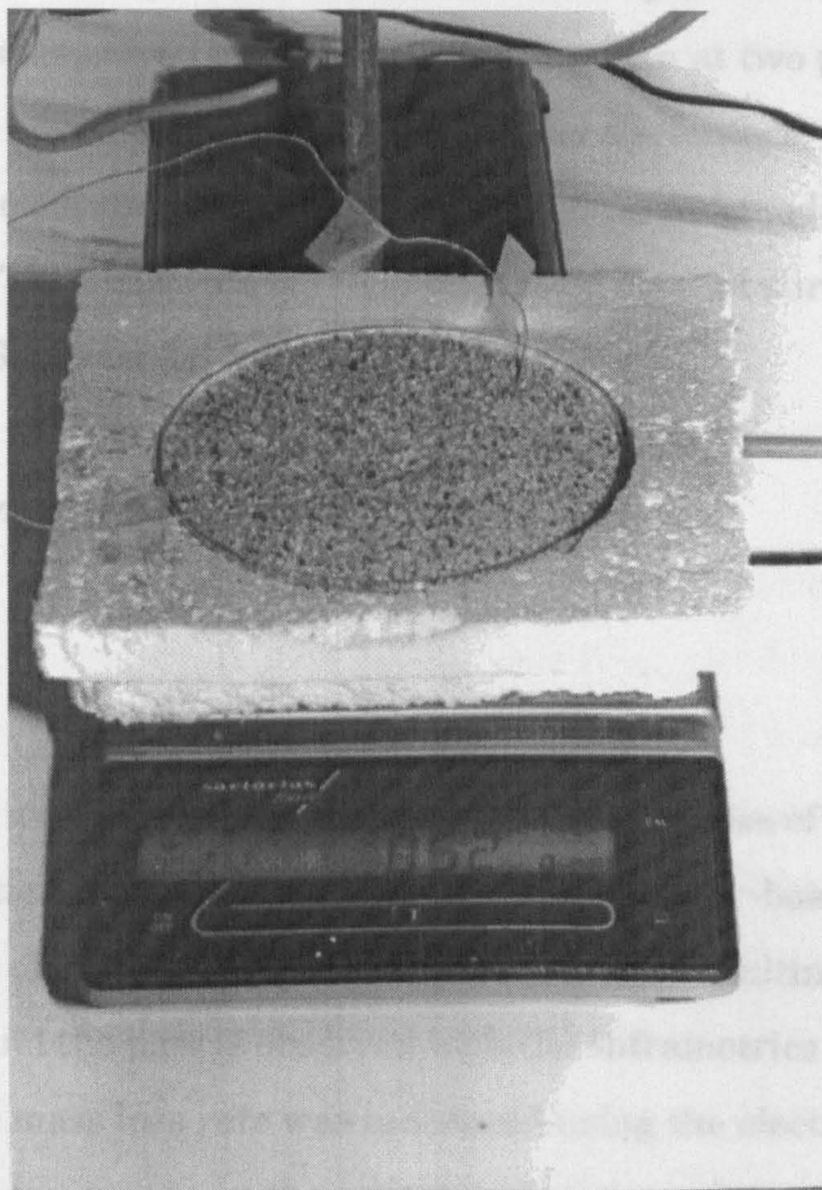
Fig. 2.8.3: Thermocouples in sand/pentane matrix. One is positioned at surface, two others are located at the bottom of the Petri dish beneath the sand.
