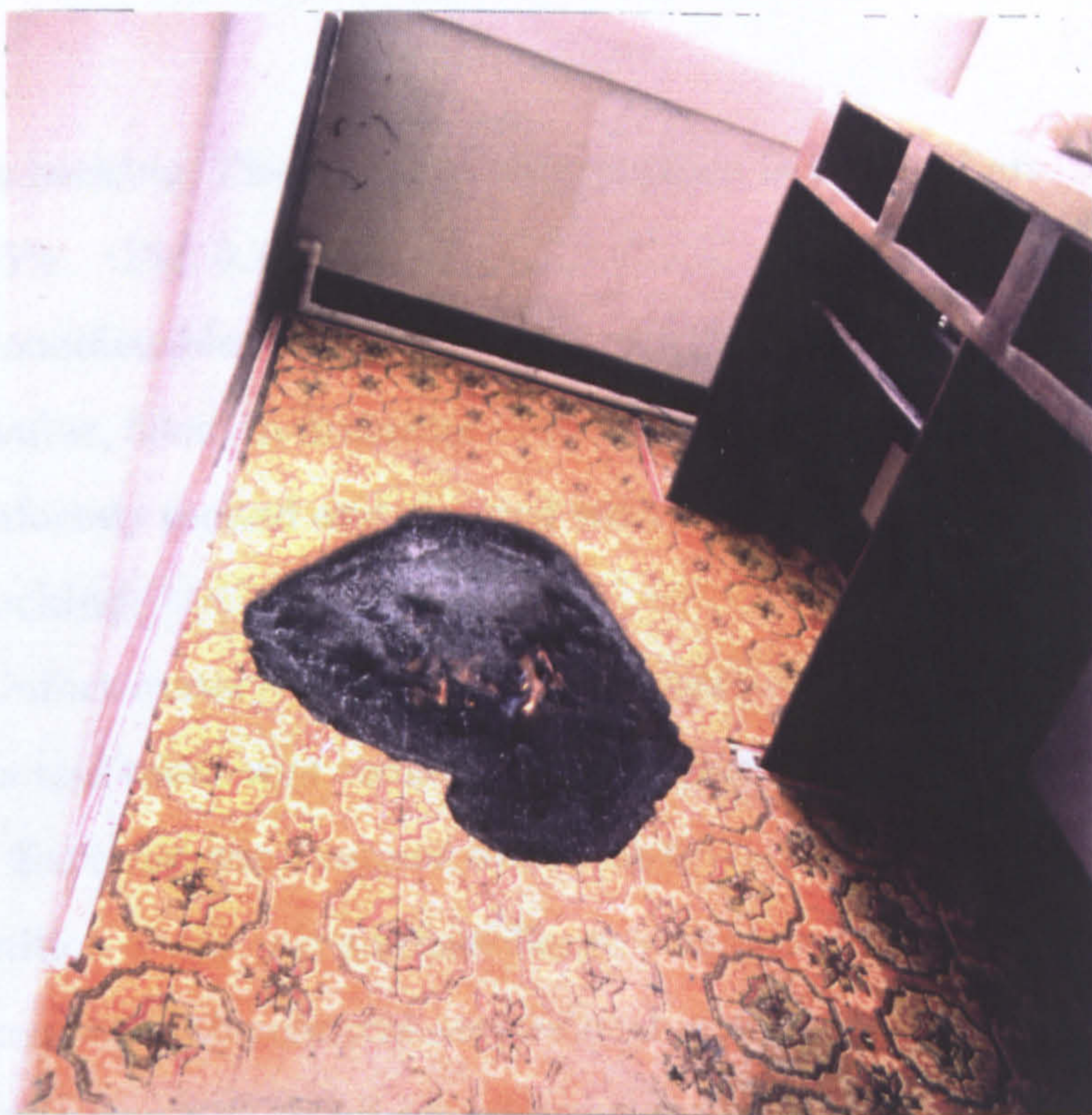
Fig. 3.10.4.1: Methanol pool on acrylic loop-pile carpet (Test 1) just as flames self-extinguish. Carpet is deeply charred at the margins of the original pool, less completely scorched across the centre, and penetrated in several isolated areas where the backing has failed.
