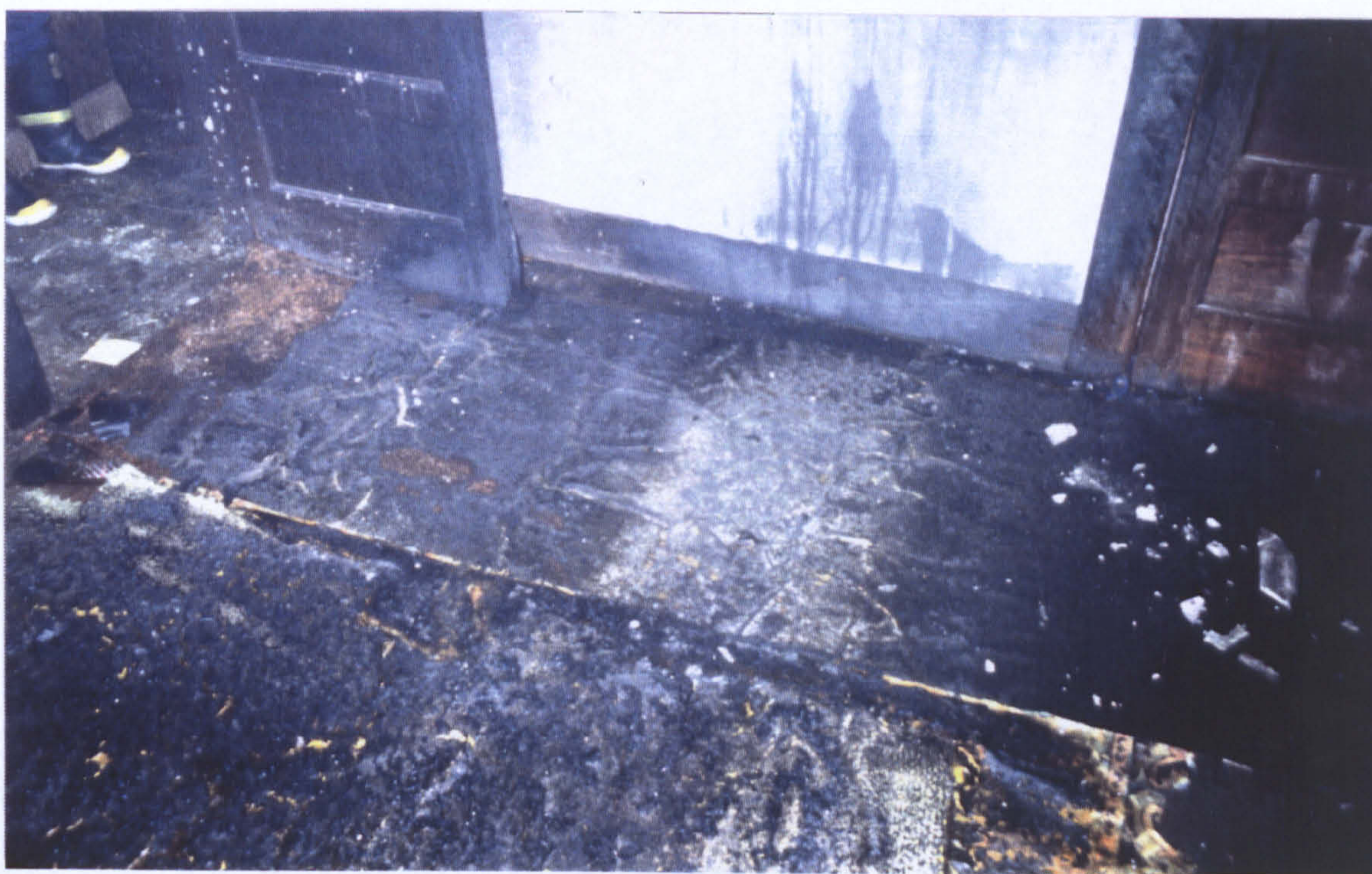
Fig. A3.10.4.16: Results of pour tests on carpet segments using 50/50 petrol/diesel fuel mixture. Burn time was approximately 5min. Large protected area in centre of rear carpet was the result of protection of carpet by wide pool (trail) of fuel. Continuous pour onto adjacent carpet segment (foreground) produced extensive destruction of carpet. Reference samples of carpet were not taken prior to test so fibre content and carpet type are unknown.
