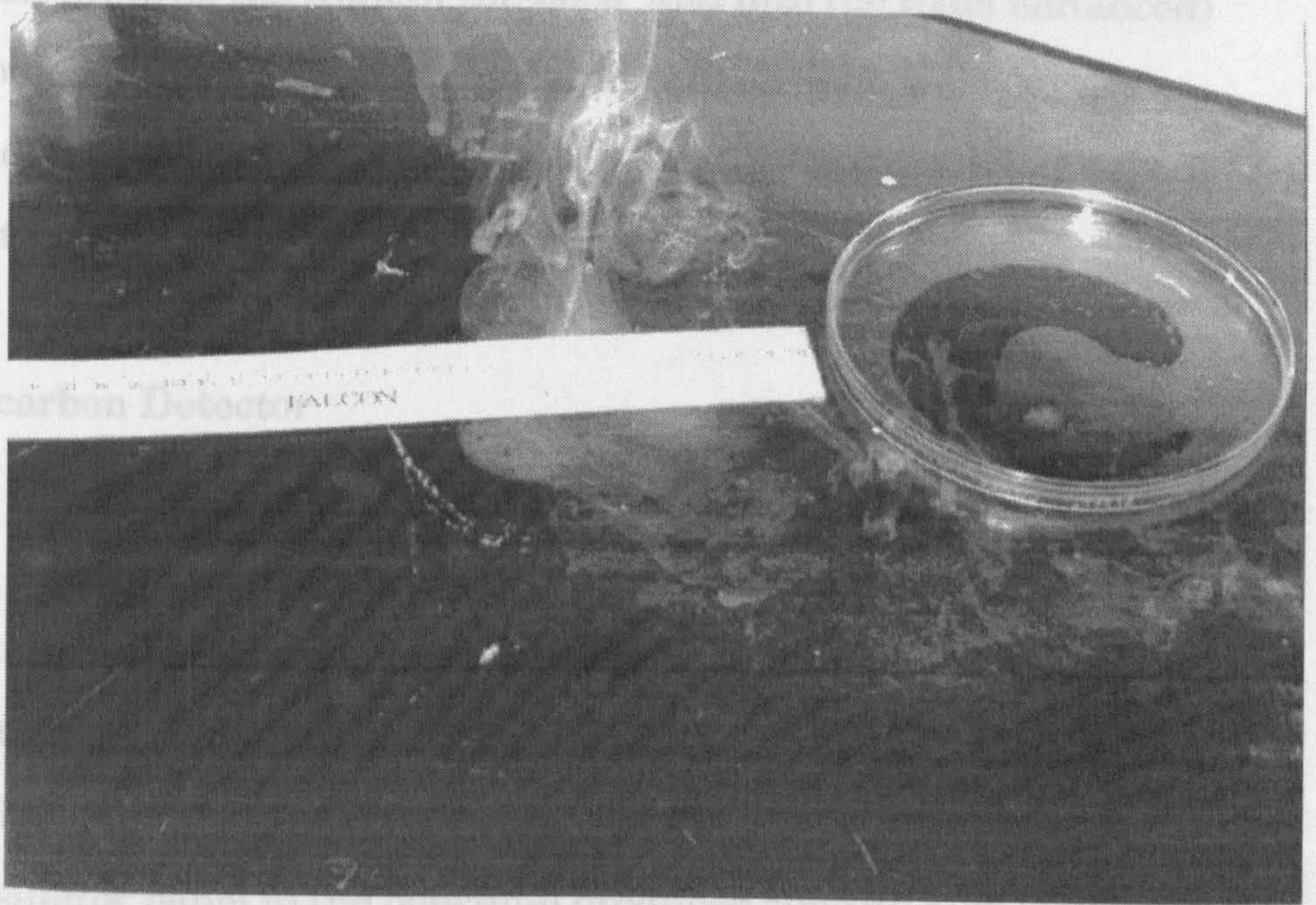
Fig. 3.7.1: Smoke pen advection test. Smoke released at edge of pan is swept along centimetre scale. Time to travel 0.3m is recorded.
