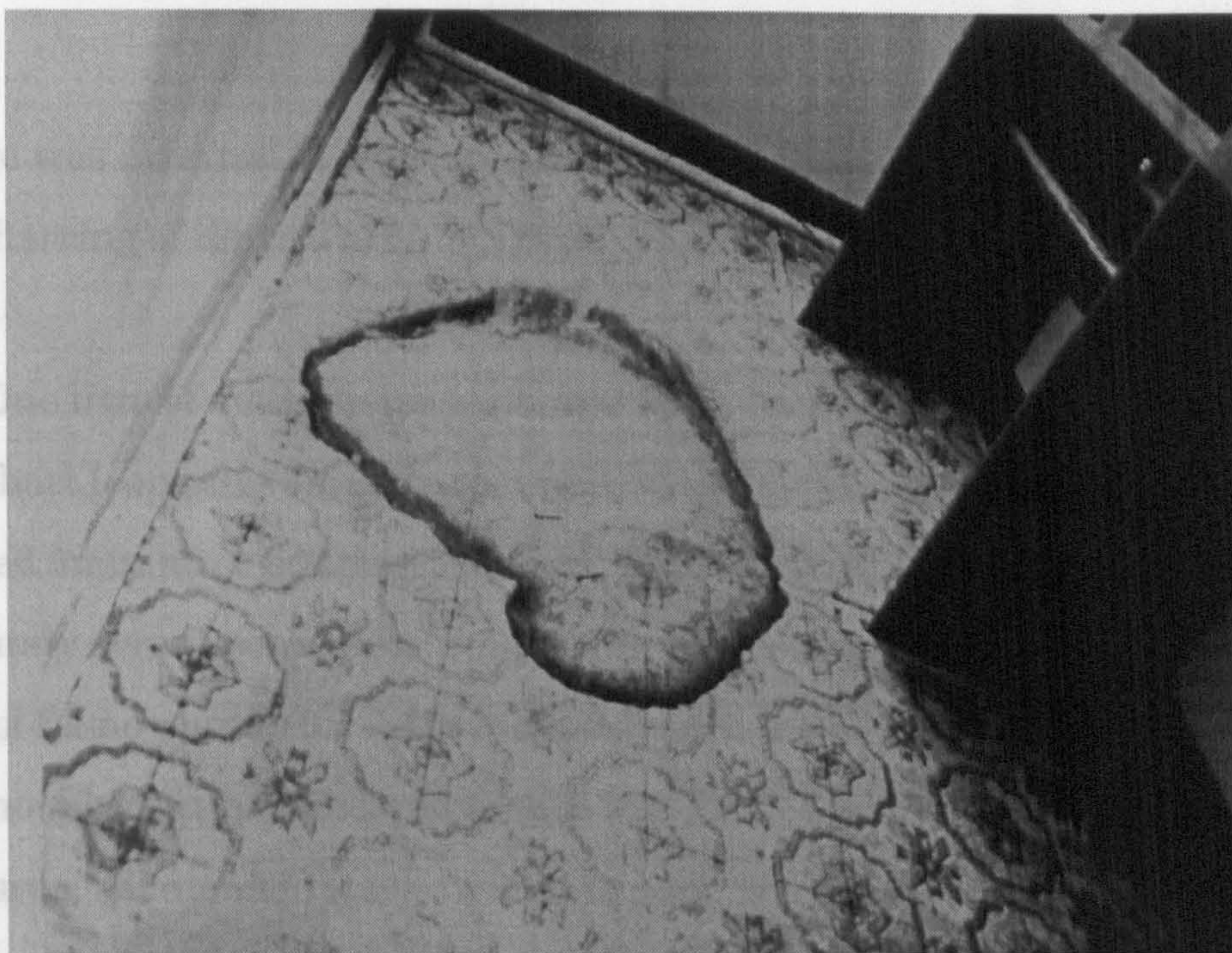
Fig. 3.10.1.1: Methanol pool fire on acrylic carpet (Test 1). Low luminosity flames are barely visible but the carpet has charred in a halo pattern around the margins of the pool. Some scorching of the carpet pile has begun in the lower right quadrant of the pool as the methanol evaporates.
