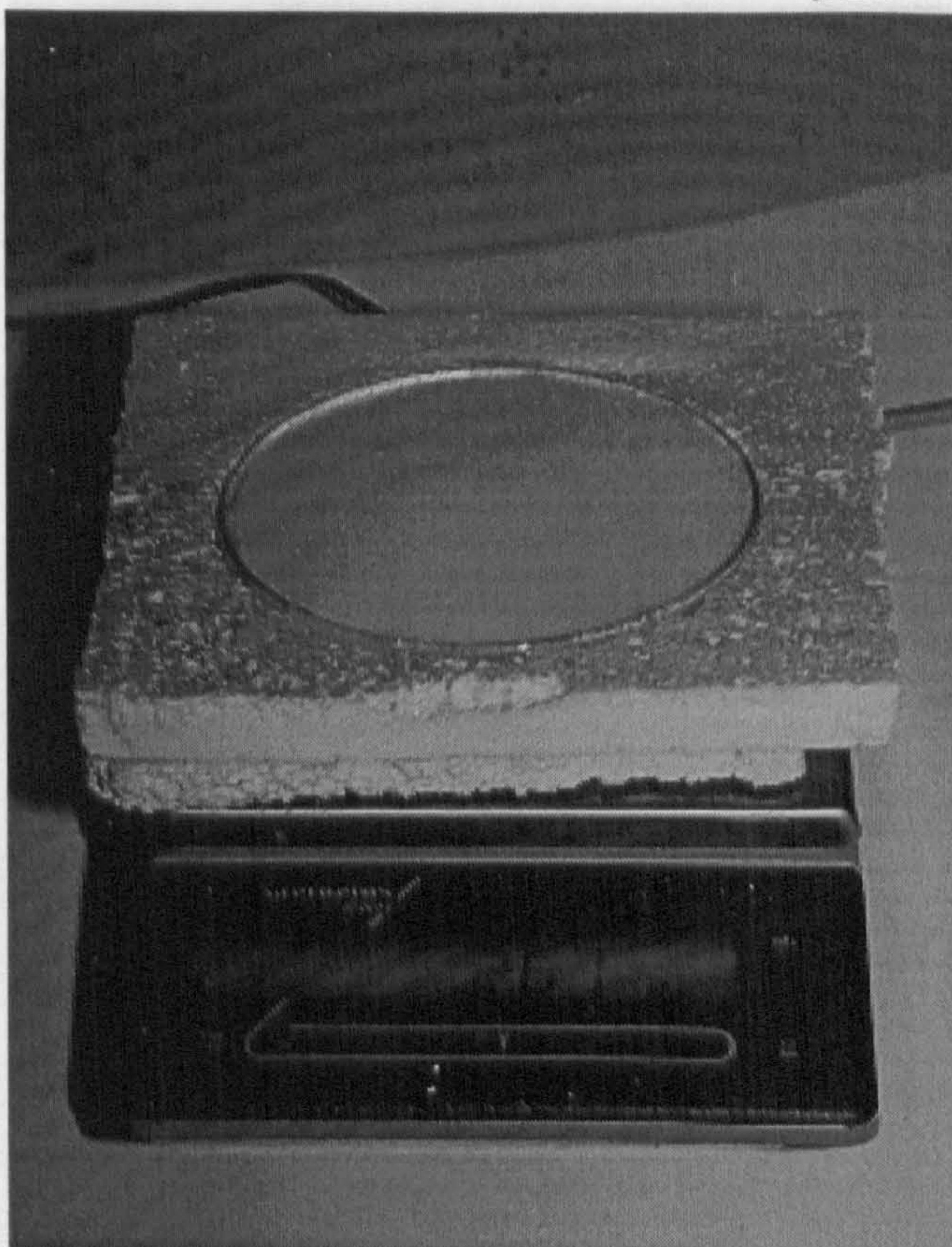
Fig. A.2.2.2.1(a): Balance with insulated Petri dish and polyurethane foam substrate.
