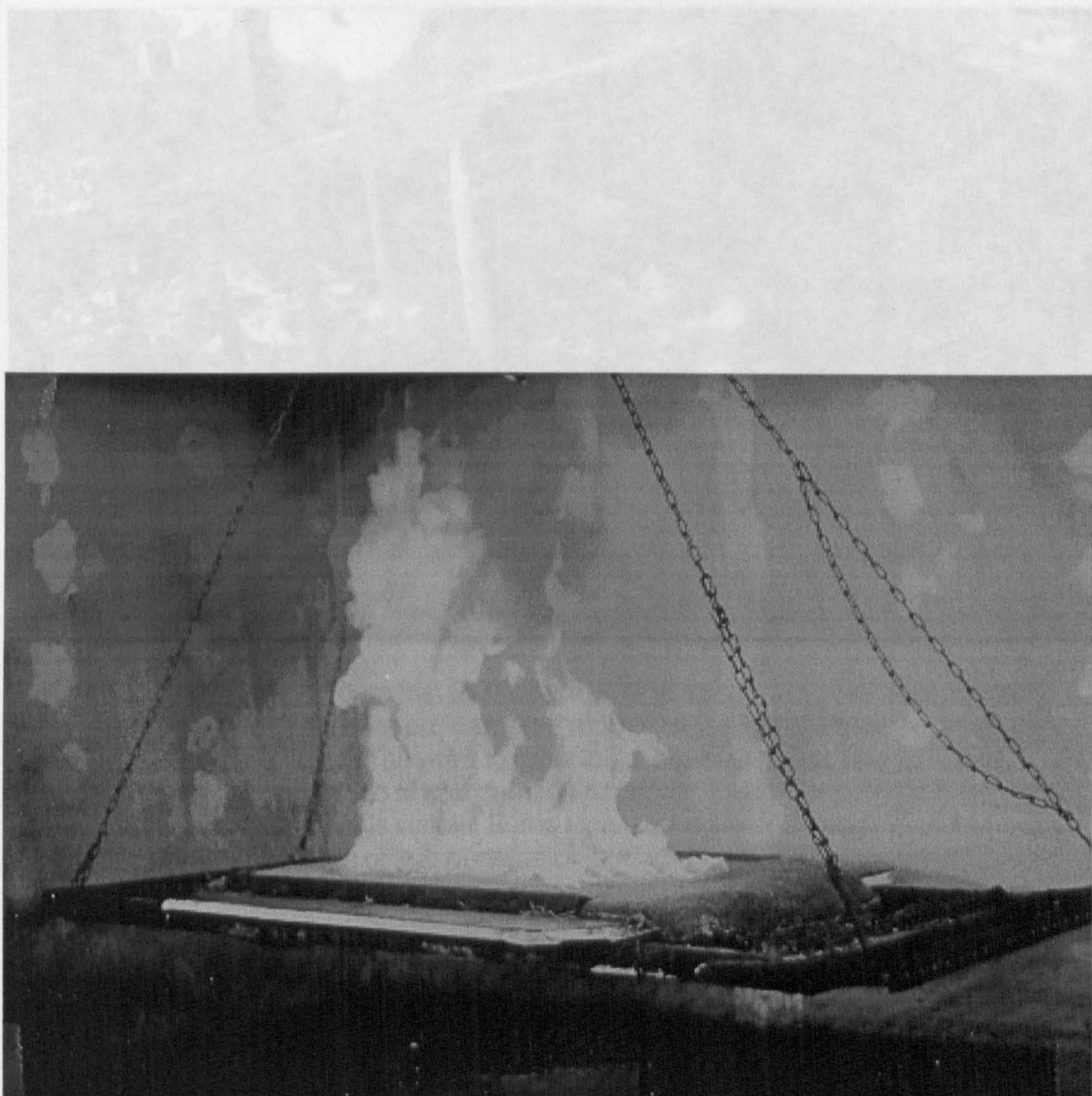
Fig. A.3.10.2.1: Typical flame plume above camping fuel on carpet (Test 10). Height estimated at 1.2m. Photo taken approx. 1min after ignition.
