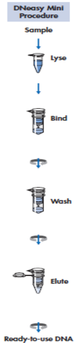
Figure 5.1 Diagram Representing the Basic Protocol of the Total DNA Isolation from the Rat Liver Tissue.
