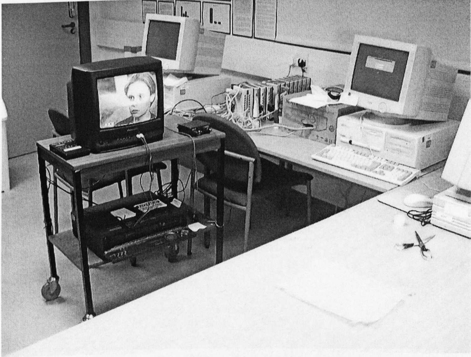
Photo 3. Psychophysiological laboratory: The acquiring equipment connected to the specially designed equipment for triggering automatically the acquisition (by pressing the start button of the VCR), the VCR from which the presentation of the stimulus film would be presented to the child (in the observation laboratory).
