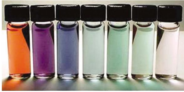
Figure 4. Visual demonstration of the tunability of metal nanoshells. From left to right the gold shell thickness decreases from 20 to 5 nm. The silica core is 60 nm for each sample. 70 Image reproduced from Loo C. et al., Technology in Cancer Research & Treatment , 2004 (open access article).
