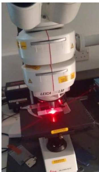
Figure 45. Photograph of a Raman microscope used for analysing LF strips.
