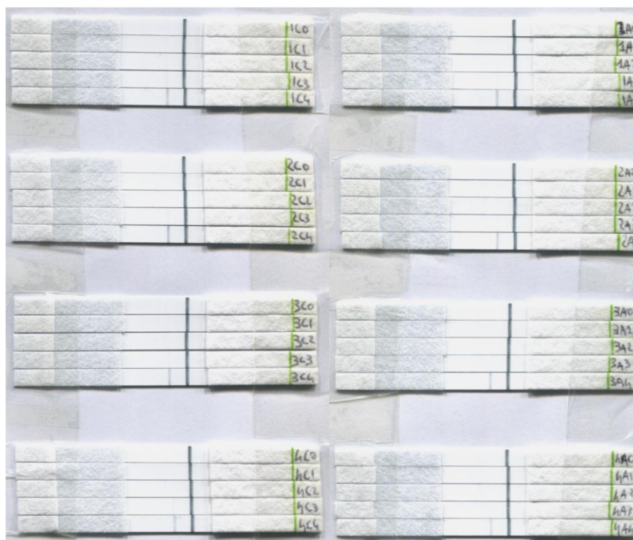
Figure Appx. F1. Scanned images of LFIA strips performed during the optimisation study. The AuNSs@MBA@anti-hCG conjugates are: 1A, 1C, 2A, 2C, 3A, 3C, 4A and 4C. Each conjugate was used to run 5 strips that contained a test line of 250 \mu\text{g}/\text{mL} of anti-hCG and a control line of 1 \text{mg}/\text{mL} of anti-mouse IgG. Sample pads were loaded with hCG as follows: 0 (blank), 1 (0.005 \text{ng}/\text{mL} ), 2 (0.05 \text{ng}/\text{mL} ), 3 (0.5 \text{ng}/\text{mL} ) and 4 (5 \text{ng}/\text{mL} ).
