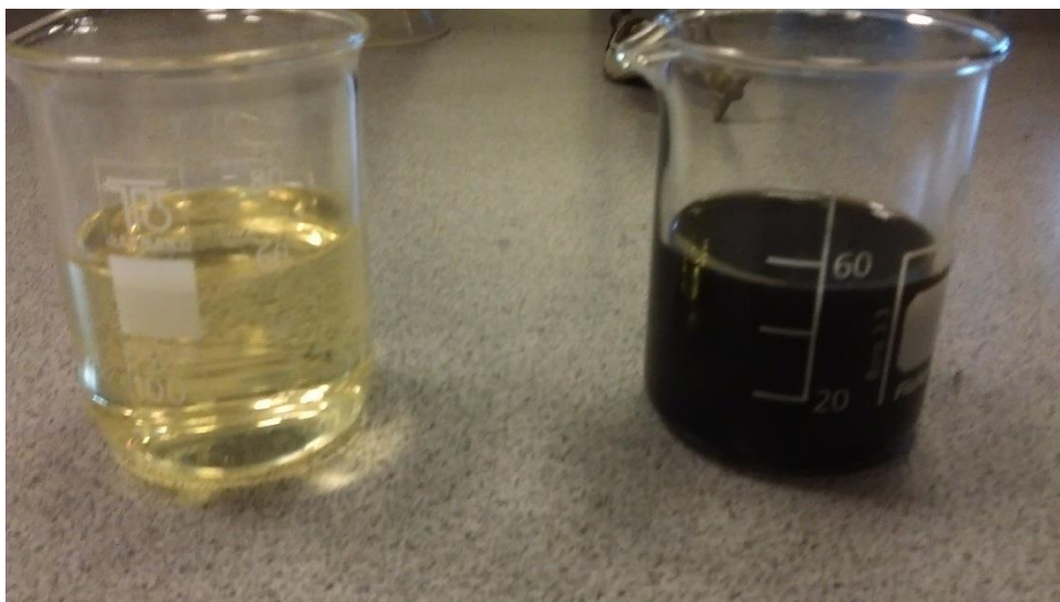
Figure 45 - Photograph of the pre-sooted engine lubricant (right) to be used in initial engine-based sorption studies (a sample of fresh lubricant is shown on the left for reference)
