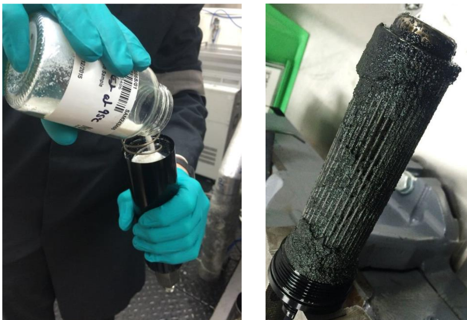
Figure 46 - Photographs of filter element and polymer particles before (left) and after (right) engine based sorption test
