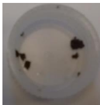
Figure 70 - Photograph of poly(styrene-co-VBC-co-EGDMA) after the 8-hour fired engine test
