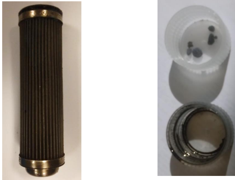
Figure 62 - Photograph of filter element after fired engine test (left) and image of poly(DVB-80-co-4-VP) after fired engine test (right)
