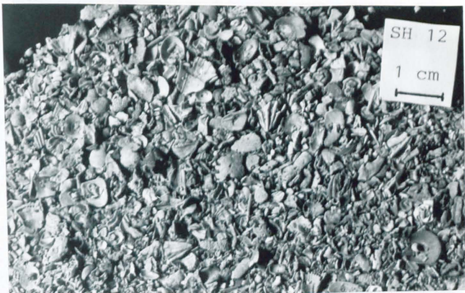
Figure 21 Typical Inner Hebridean carbonate, rich in bivalve and barnacle debris. Rubha Nan Clach deposit (see Fig. 32a).
