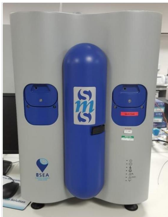
Figure 3-11: The inverse Gas Chromatography-Surface Energy Analyzer (iGC-SEA).
