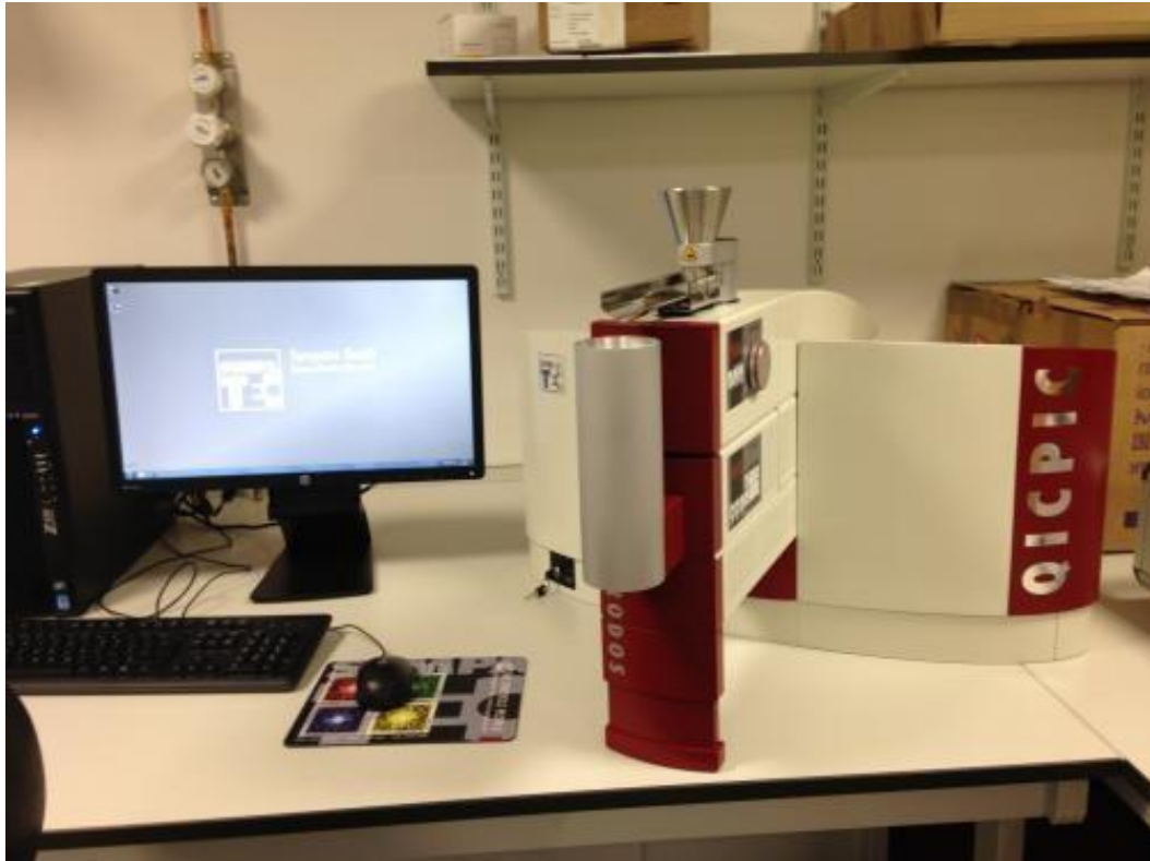
Figure 3-1: The QICPIC ® – RODOS dynamic image analysis instrument.
