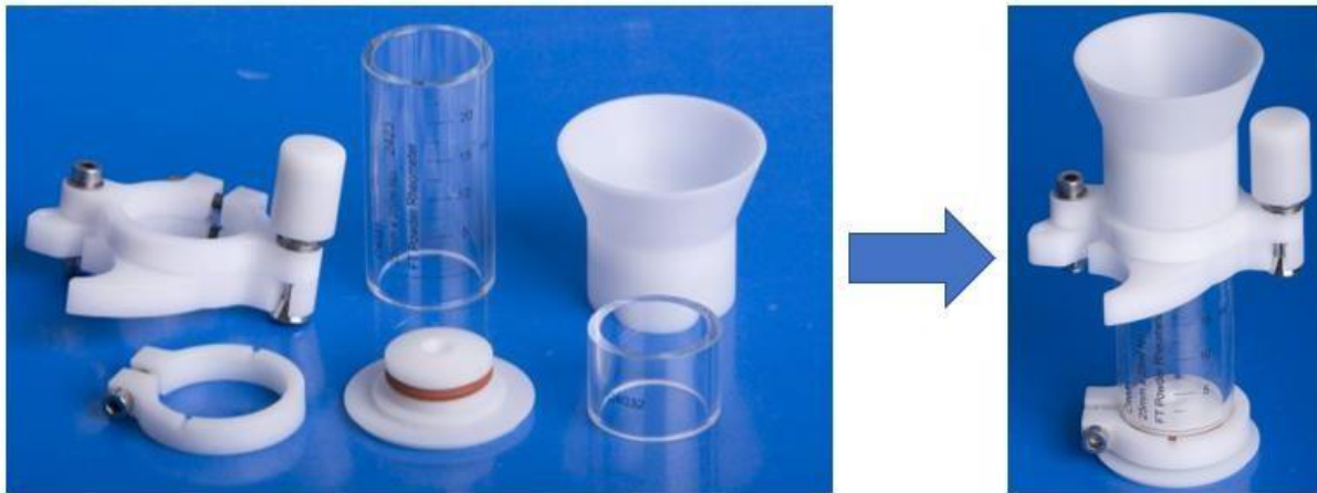
Figure 3-12: The 10 ml x 25 mm split vessel used to carry out the powder flow measurement.
