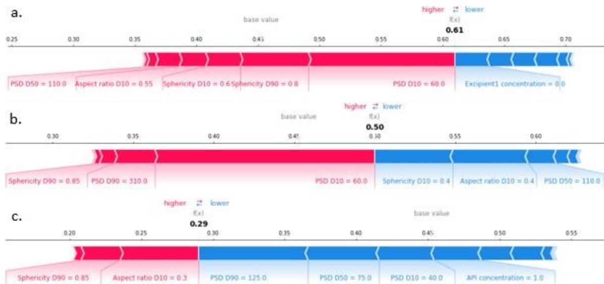
Figure 4-45: Flowability predictions for Materials 1 (a), 2 (b), and 3 (c) . Variables that increased the probability of being free-flowing were presented in pink, and variables that decreased the probability of being free-flowing were presented in blue. The length of the bars of the variables represented how much the variables impact the model outcome.
