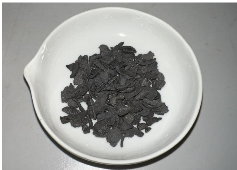
Figure 4.9: Example of Biochar Material Produced in This Study
