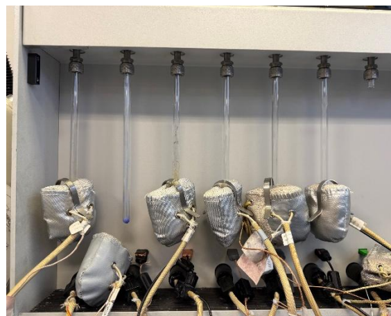
Figure 4.19: Samples Undergoing Degas on Degas Ports
