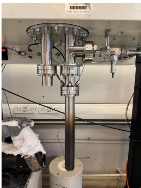
Figure 4.35: IGA with Sample Chamber Attached
