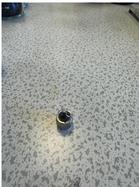
Figure 4.37: Sample Bulb Filled with Biochar Sample
