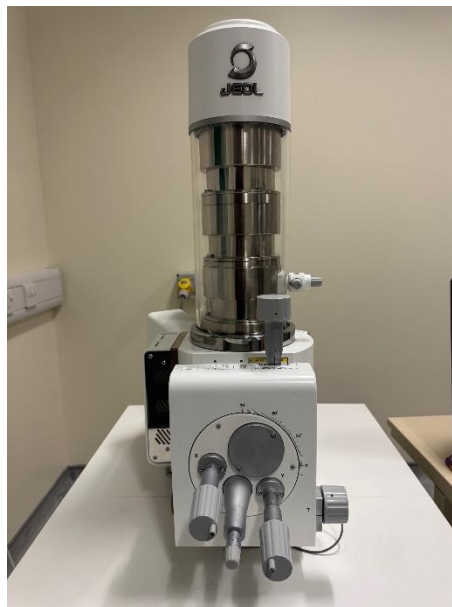
Figure 4.31: JEOL JSM-IT100 SEM (Sample Movement Handles Can Be Seen Extending from the Equipment)
