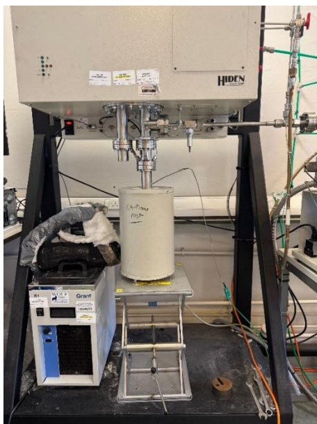
Figure 4.39: Furnace Attached to IGA Sample Chamber
