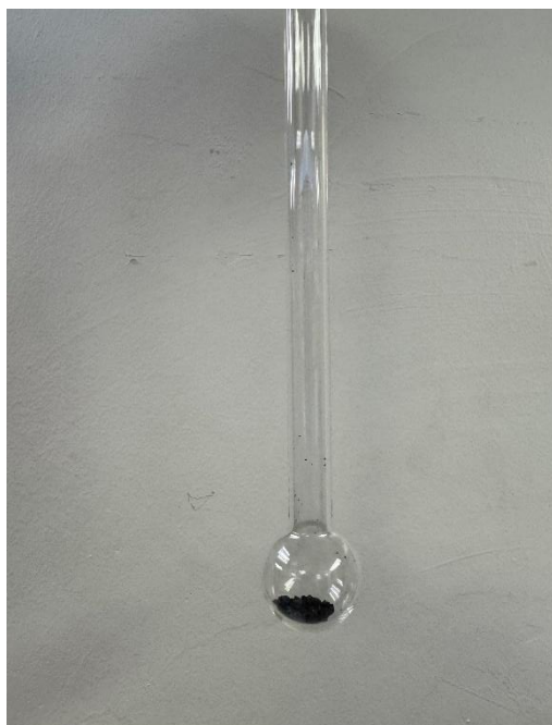
Figure 4.18: Biochar Sample in BET Tube
