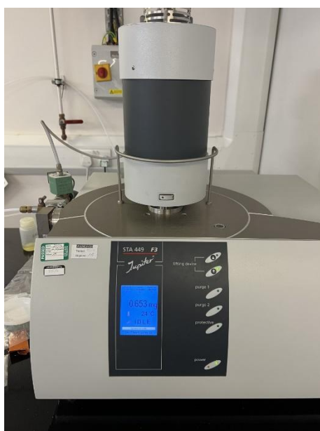
Figure 4.21: NETZSCH STA 449 F3 Jupiter System Used in This Study
