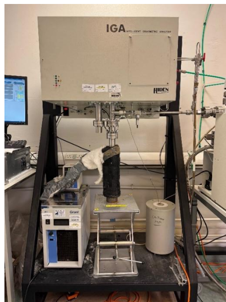
Figure 4.40: Water Bath Attached to IGA Sample Chamber
