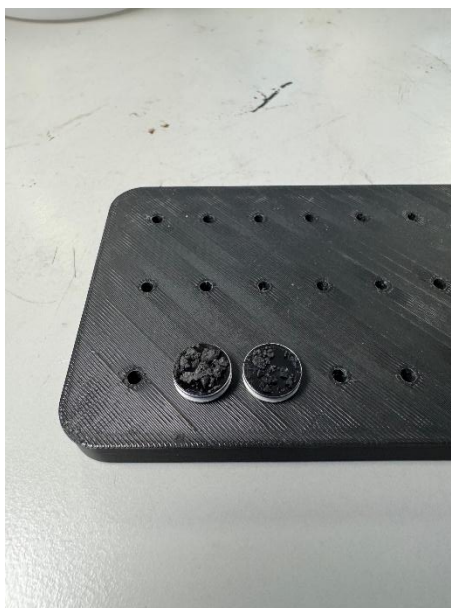
Figure 4.28: Example of Biochar Attached to SEM Stubs using Carbon Tape
