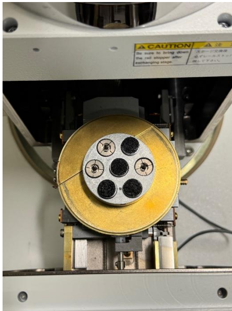
Figure 4.29: Multi-Sample Holder Used in JEOL SEM
