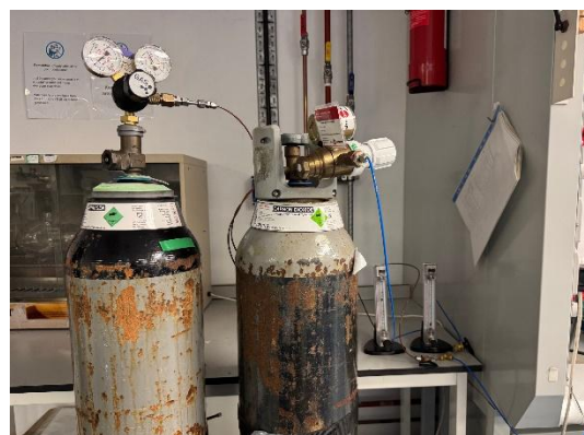
Figure 4.8: Gas Cylinder Setup Connected to Lenton Furnace
