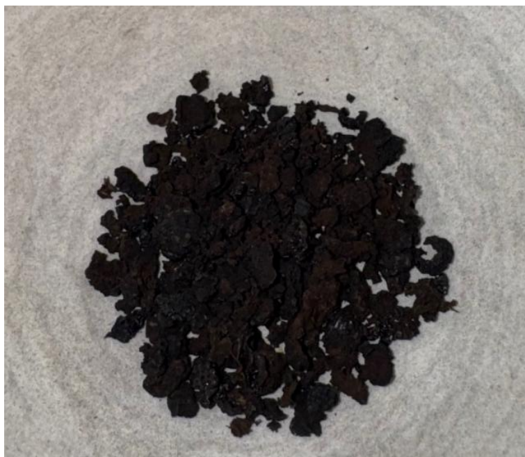
Figure 4.16: Example of Hydrochar Material Produced in This Study
