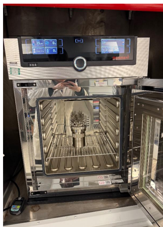
Figure 4.14: Autoclave Inside Memmert UF55 Plus Oven
