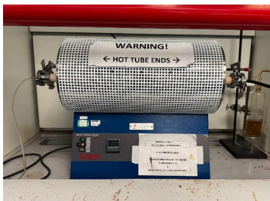
Figure 4.7: Lenton Tube Furnace
