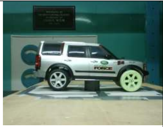
Figure 7.7 Model with ground board in place
