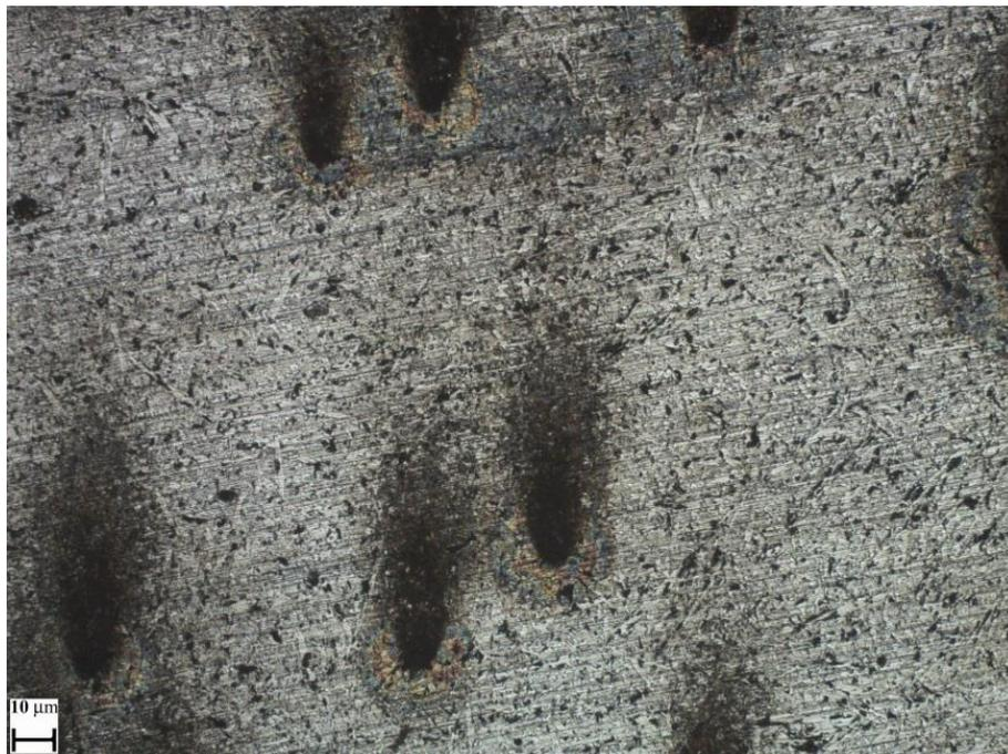
Figure 8.46: Pitting corrosion on 30WCI at 10% NaCl.
