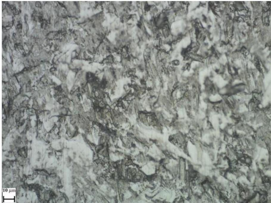
Figure 8.43: Microscopic view of 38WCI OA at 10% NaCl.
