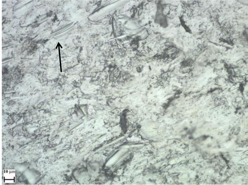
Figure 5.19: UNS S31600 OA at pH 3 after 1h SLEC test – abrasive markings (arrow).
