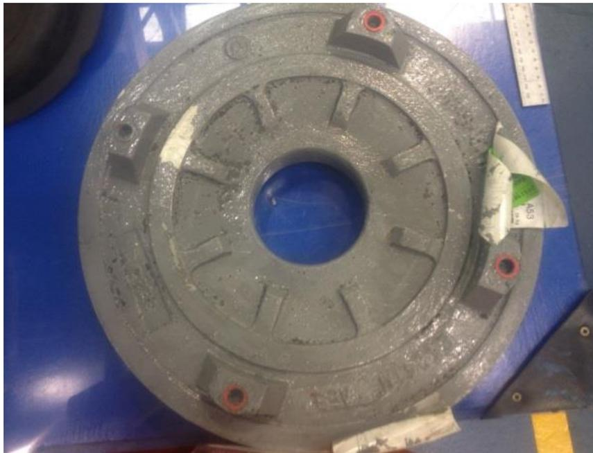
Figure 4.2: 37WCI frame plate liner insert (diameter 430 mm, thickness 35 mm).
