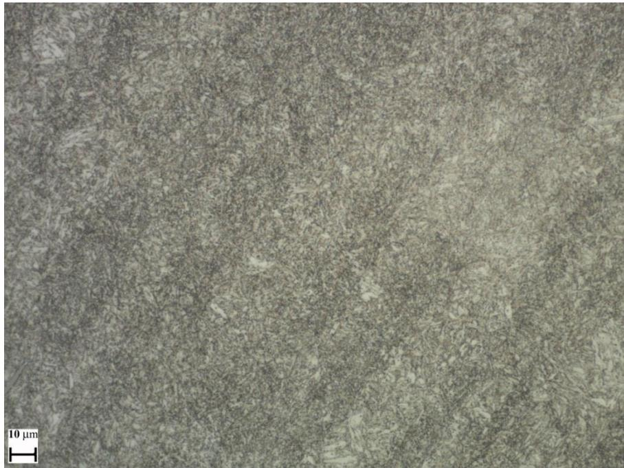
Figure 5.2: Microstructure of UNS S42000 [etched].
