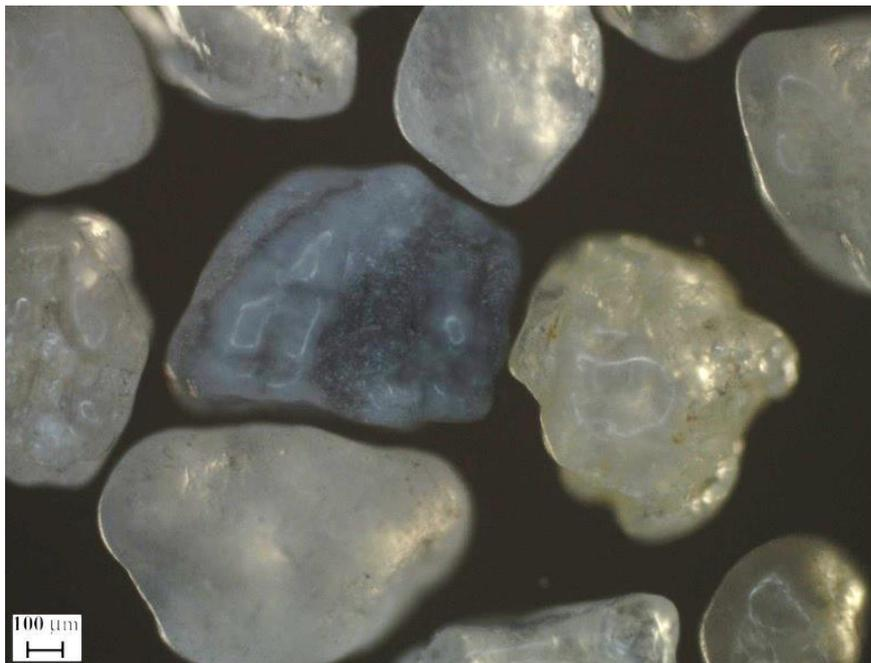
Figure 4.3: Microscopic view of the angular shape of silica sand.
