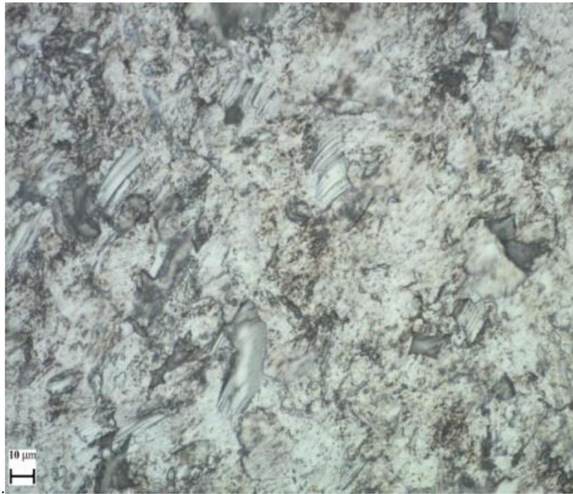
Figure 5.32: UNS S42000 OA at pH 7 after 1h SLEC test.
