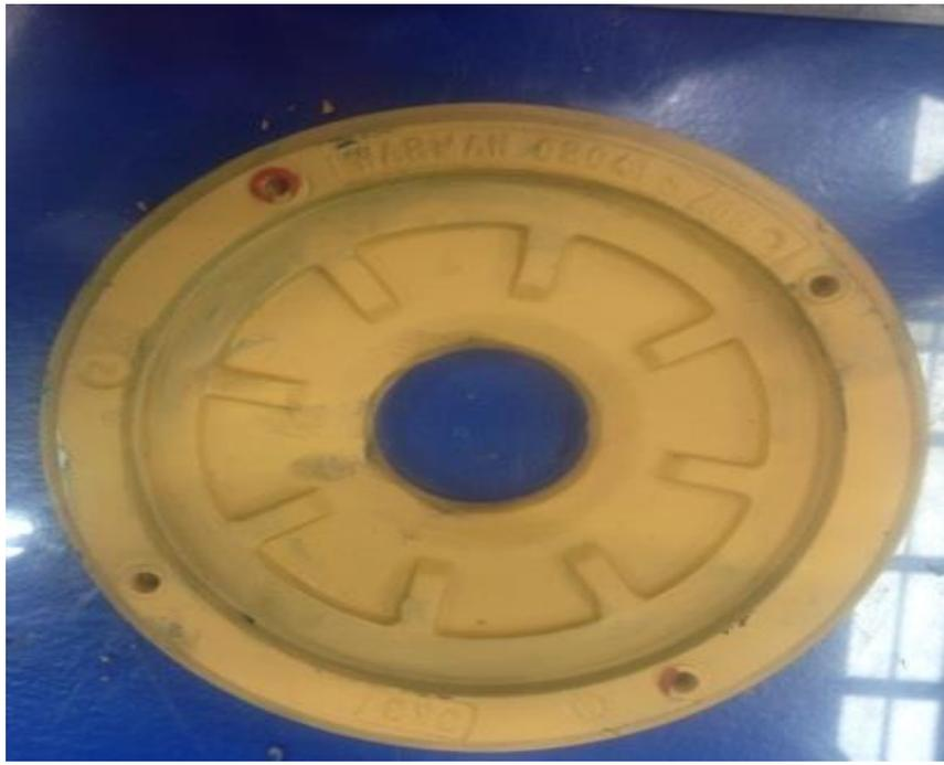
Figure 4.1: 27WCI frame plate liner insert (diameter 200 mm, thickness 30mm).
