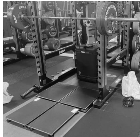
Figure 9. Set up for a traditional back squat when performing the movement on PFPs.
