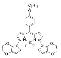
**13** (250 mg, 0.4 mmol) was dissolved in dry dichloromethane (25 mL) and triethylamine (0.2 mL) was added. The reaction was stirred for 30 min and boron trifluoride diethyl etherate (1 mL) was slowly added. The reaction was stirred at room temperature under nitrogen overnight. The reaction mixture was washed with
