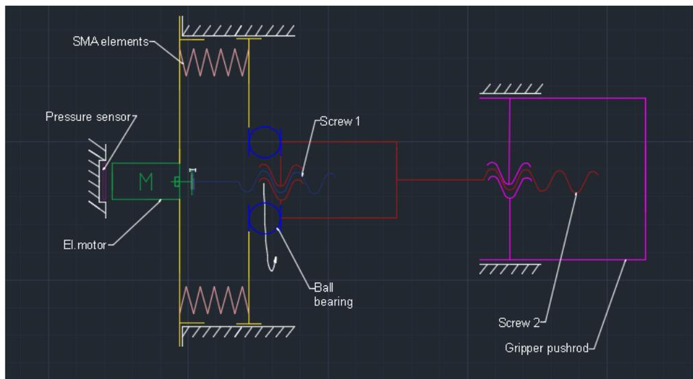
**Figure 10.** Schematic look of developed actuator design
