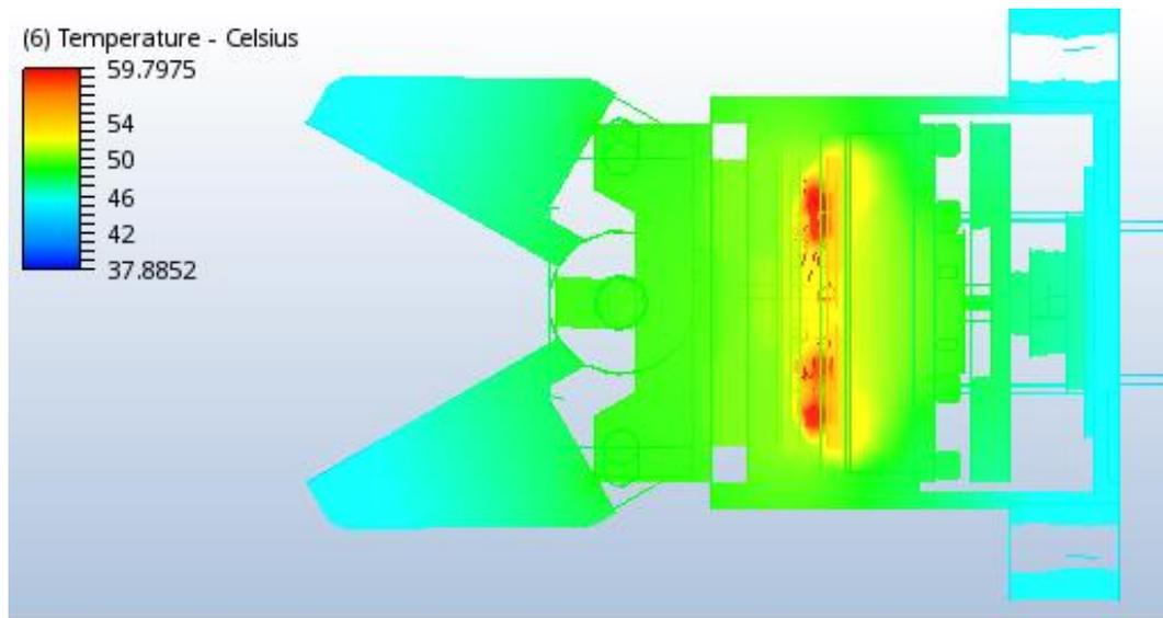
**Figure 25.** Device inner elements steady state temperature map
