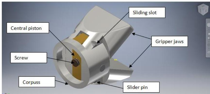
**Figure 8.** Gripper CAD model
