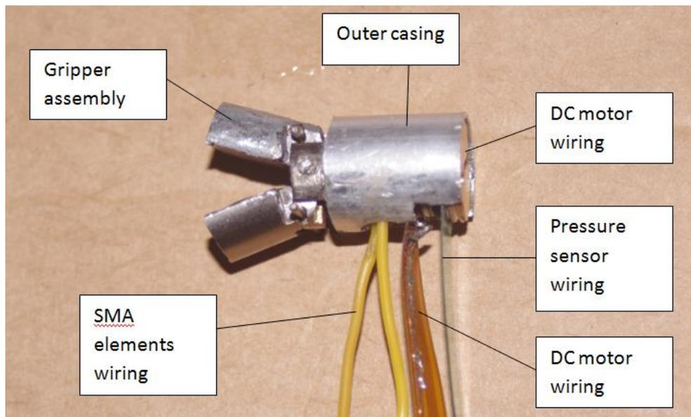
**Figure 30.** Fully assembled prototype
