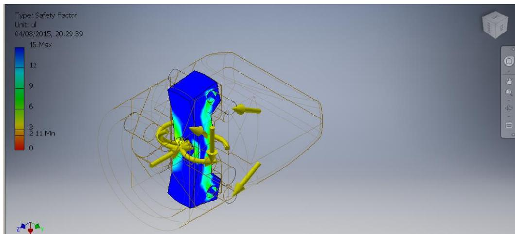
**Figure 9.** Gripper critical component strength analysis results
