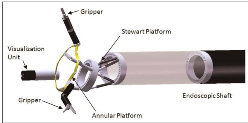
**Figure 2.** Robotic system design for minimal access surgery [11].
