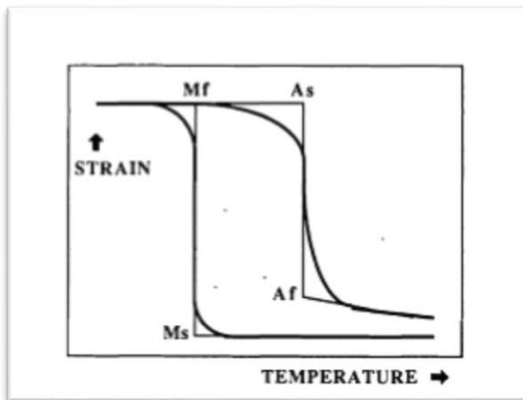
**Figure 5.** Typical SMA phase change curve
