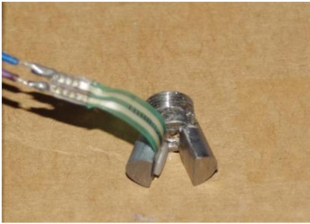
**Figure 30.** Gripper assembly with mounted force sensor
