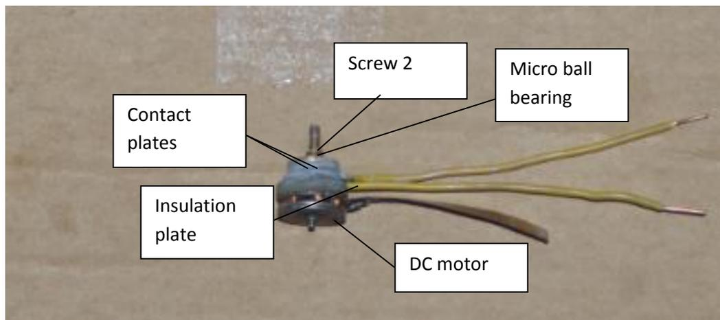
**Figure 29.** Hybrid actuator assembly
