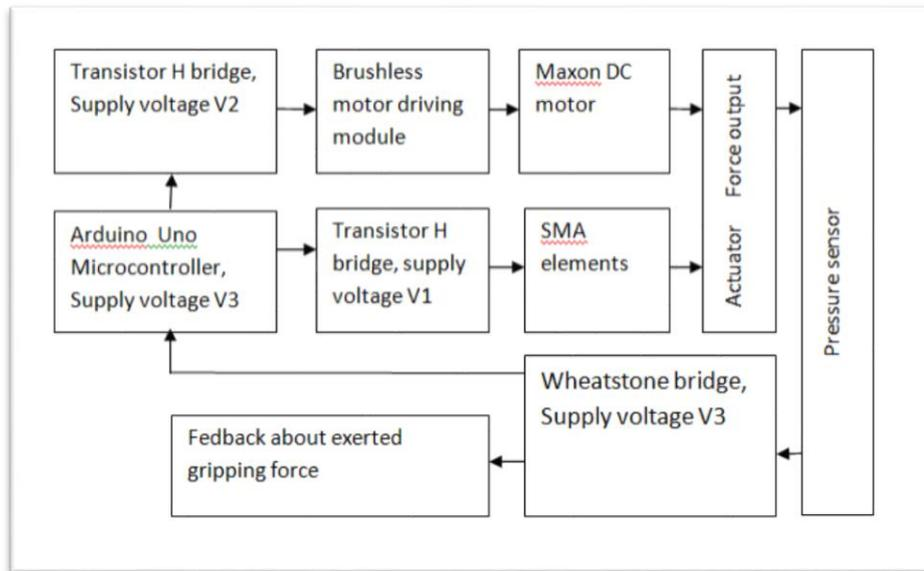
**Figure 21.** Block diagram of device control system
