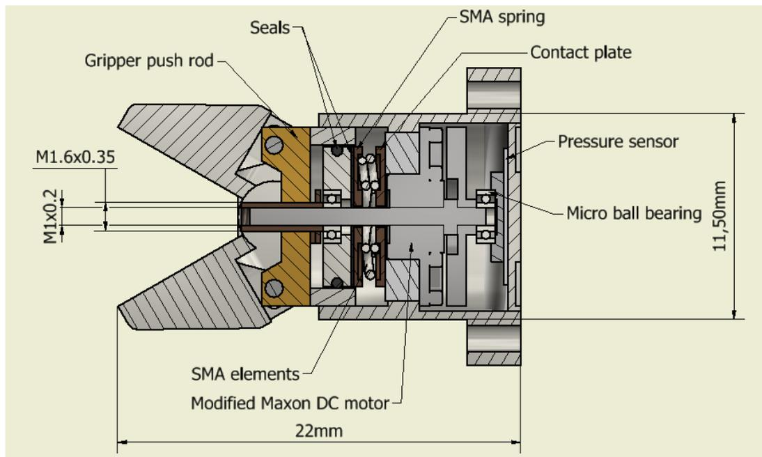
**Figure 22.** Device design sectional view
