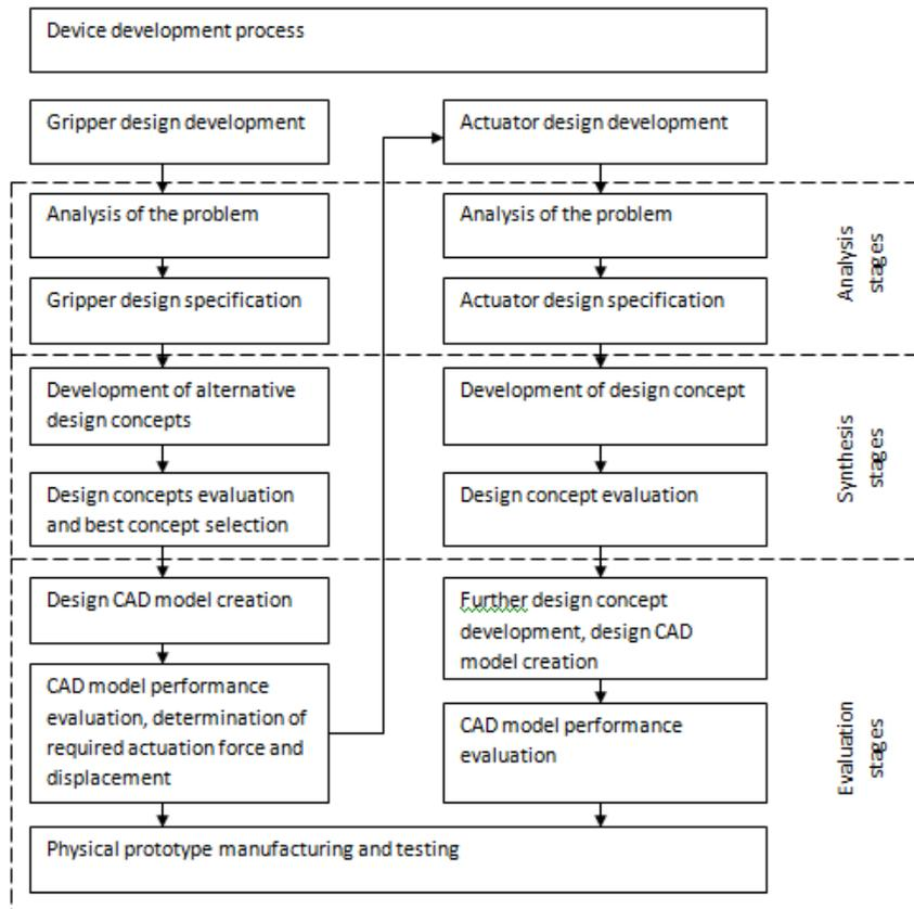
**Figure 6.** Design process flow chart
