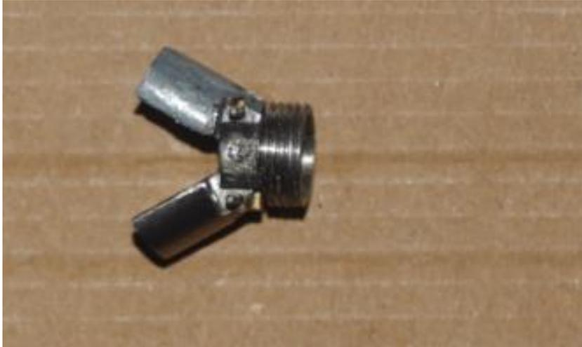
**Figure 27.** Gripper assembly
