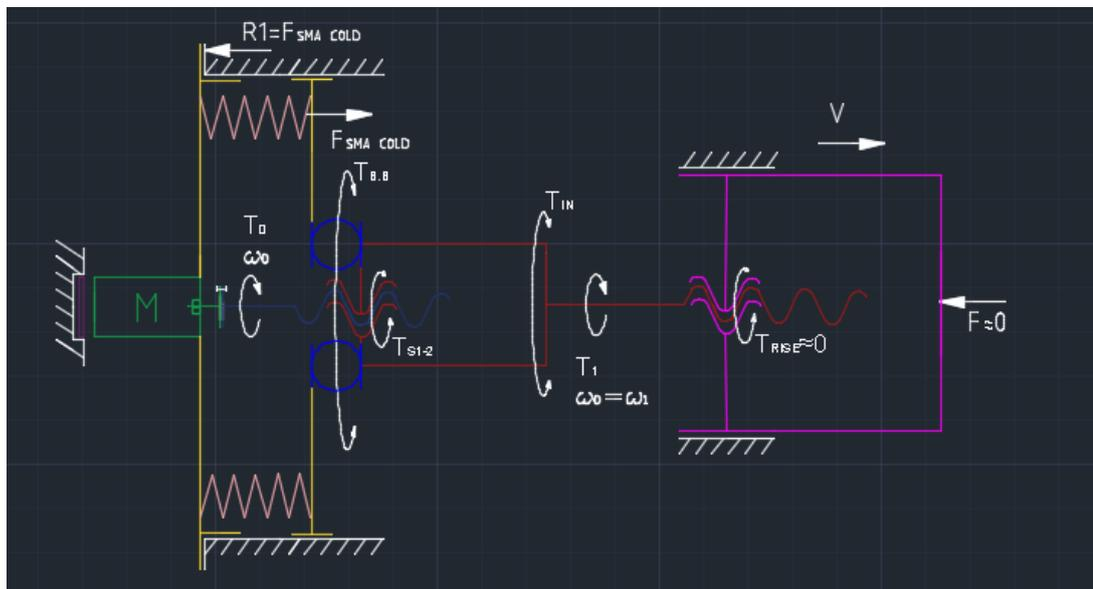
**Figure 12.** Actuator operation, Event F1
