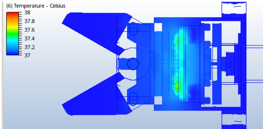
**Figure 26.** Temperatures of device internal elements after 5s from inactivation
