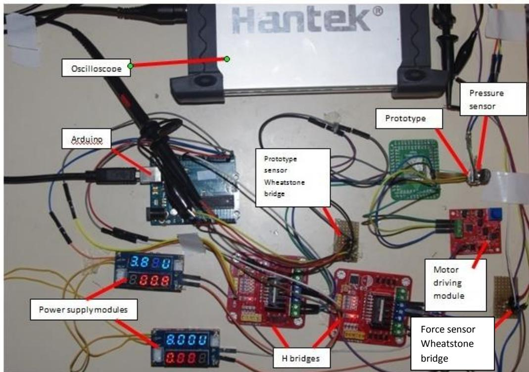
**Figure 31.** Prototype testing setup
