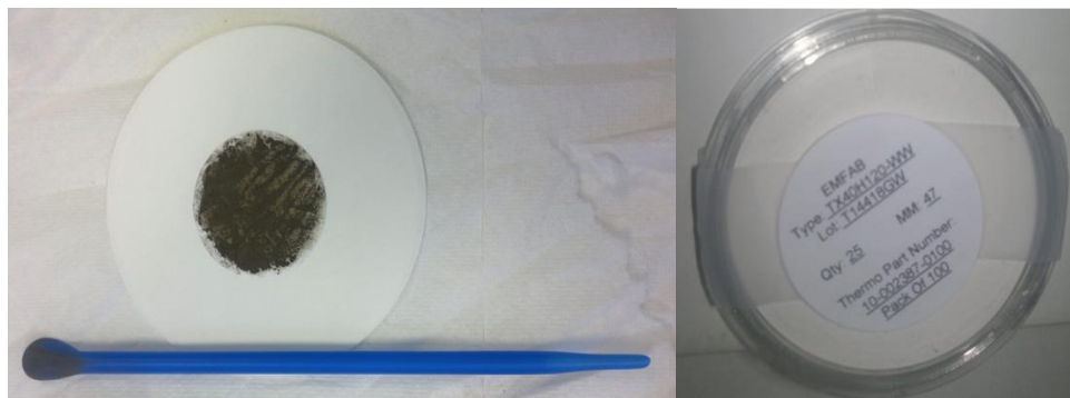
Figure 3.1. Blank and loaded Pallflex TX40 FDMS filters
