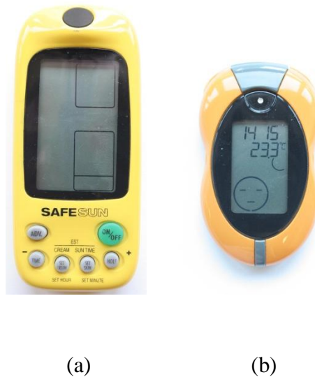
Figure 1. 5 A picture of (a) a SunSafe™ and (b) an NSecssity personal UV meter.
