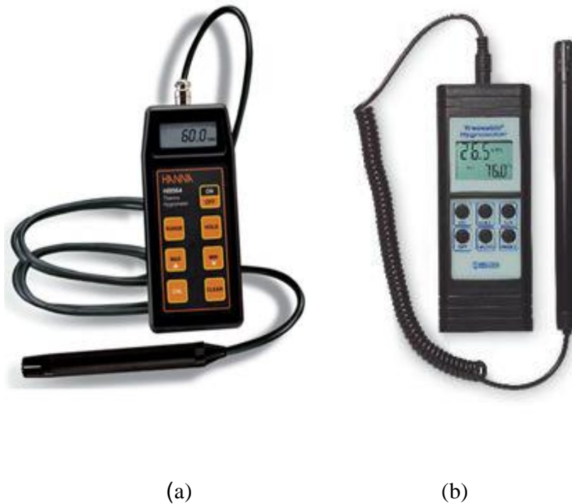
Figure 1.16 Electronic humidity sensors (a) capacitive and (b) resistive hydrometers.
