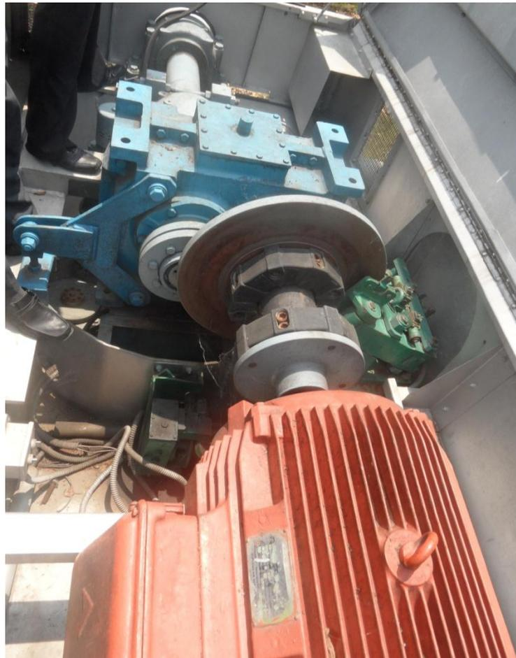
Figure 1.13 - High Speed Drivetrain, Gearbox (Blue), Generator (Red), Brake Calliper (Green)
