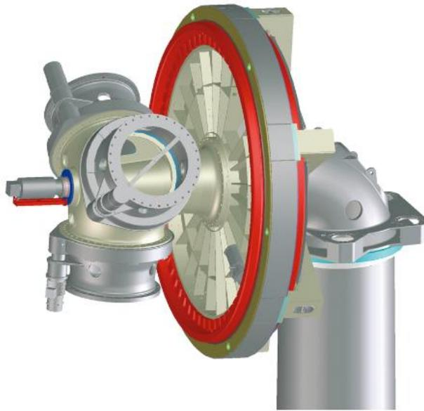
Figure 1.14 - Direct Drive drivetrain from Enercon E-48
