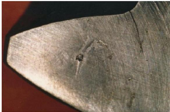
Figure 1.41 - Crack at Root of Tooth Due to Bending Moments [1.38]
