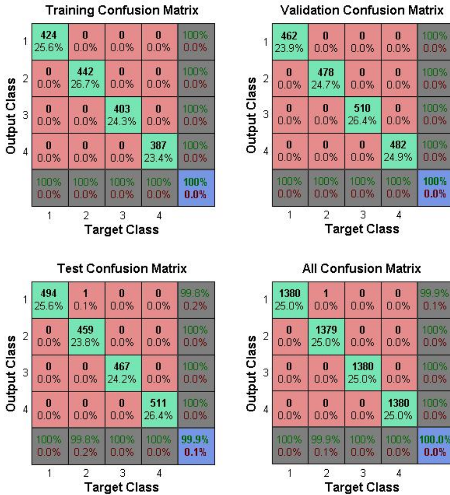
Figure 8.54: Resulting Confusion Matrix in the Flexor Muscles - S2 - Confusion matrix from the different stages of the supervised machine learning, i.e. training; validation; testing; and the summation of all the previous. The accuracy of the classification is shown for each case. For the testing, the accuracy was 99.9% with a 0.1% of classification error. For the flexor muscles, it is not clear which position is mostly a false classification.
