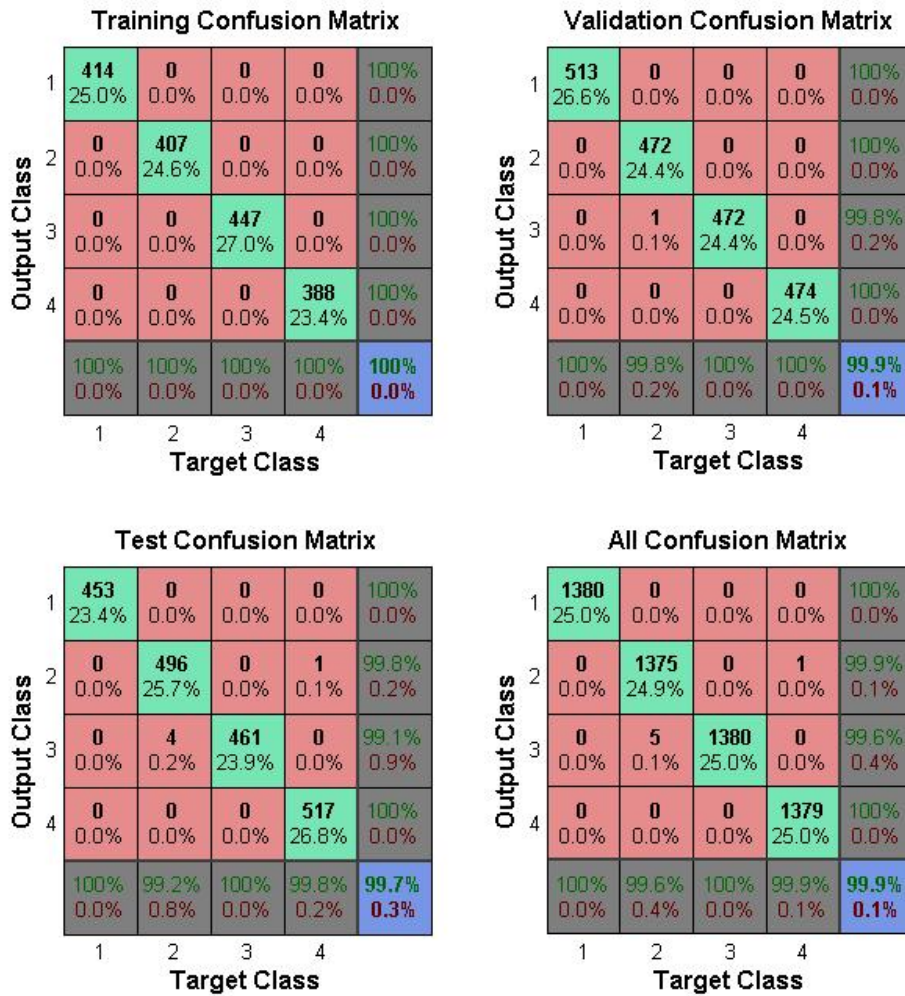
Figure 8.55: Resulting Confusion Matrix in the Extensor Muscles - S2 - Confusion matrix from the different stages of the supervised machine learning, i.e. training; validation; testing; and the summation of all the previous. The accuracy of the classification is shown for each case. For the validation, the accuracy was 99.9% with a 0.1% misclassification, for the training, it was 99.7% against 0.3%.
