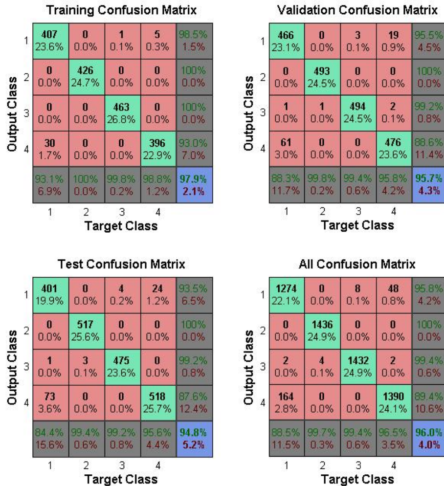
Figure 8.57: Resulting Confusion Matrix in the Extensor Muscles - S3 - Confusion matrix from the different stages of the supervised machine learning, i.e. training; validation; testing; and the summation of all the previous. The accuracy of the classification is shown for each case. For the training classification, the accuracy was 97.9% with a 2.1% of misclassification; the validation accuracy is 95.7% with 4.3% of misclassification; the test accuracy was 94.8% with 5.2% misclassification; and finally, the overall results for the muscles of the forearm was 96% accuracy with 4% of misclassification.
