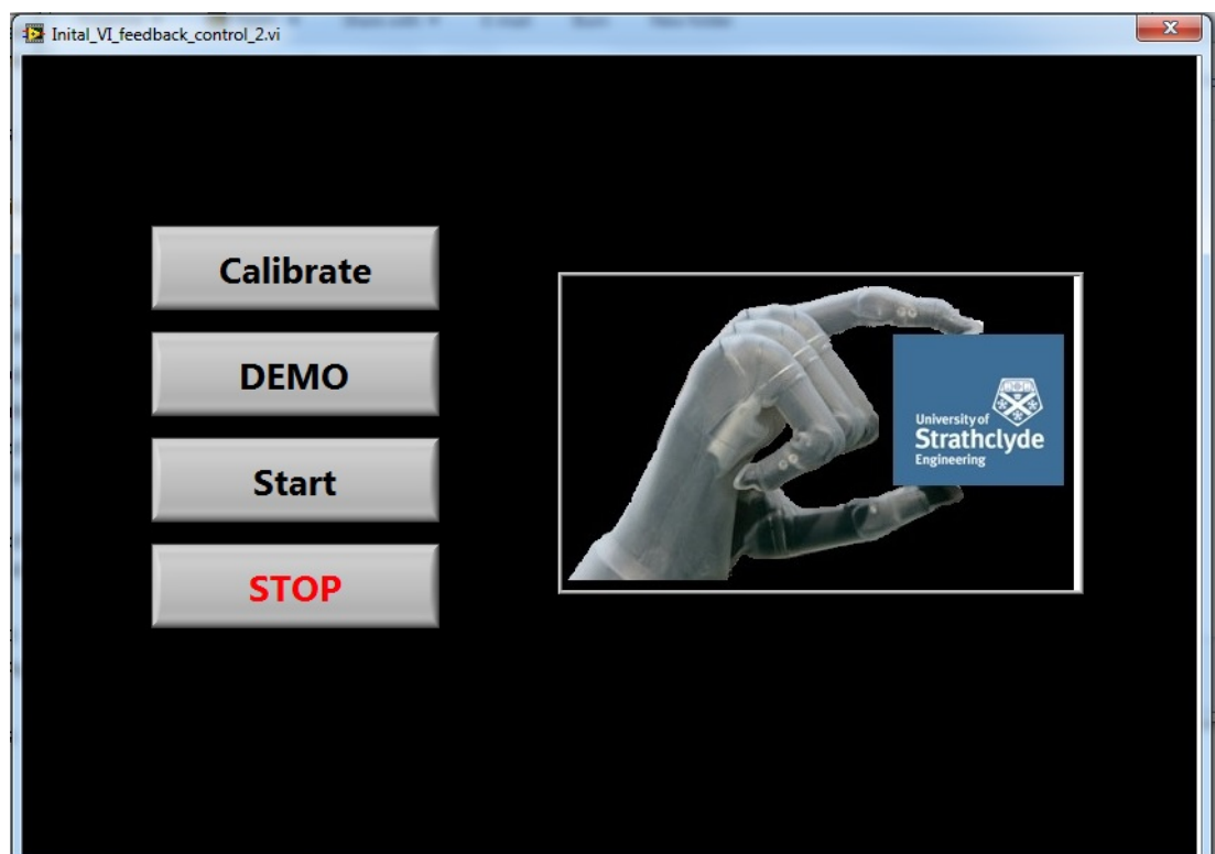
Figure 4.6: Main Menu for the Test Developed in LabVIEW - Front panel of the main menu developed for the test. This menu called up three interfaces: 1) Calibration, 2) Demo, and 3) Thumb opposition acquisition routine.
