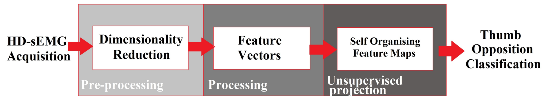
Figure 4.12: Block Diagram for HD-sEMG Feature Recognition - Block diagram representing the process for HD-sEMG thumb position classification.
