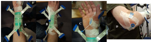
Figure 6. Electrode array matrices fixed onto the muscles. A) 64-electrode array on the extrinsic hand muscles, corresponding to the anterior compartment of the forearm. B) 64 - electrode array on the extrinsic hand muscles, posterior compartment of the forearm and 8-electrode array on the DOI muscle. C) Low-density electrode on FPB. D) Ground electrodes fixed onto the olecranon.
