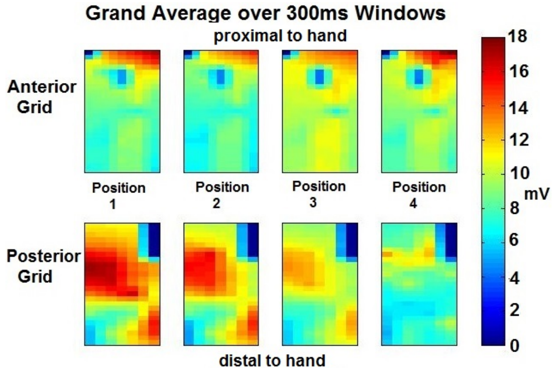
Figure 5.9: Averaged Windows for Feature Extraction per Position - The RMS values obtained during 11 windows of the IVC are averaged for each position of the thumb per grid placed on the forearm. From the anterior grid (top 4 images) a different amplitude exertion is appreciated towards the fingers, for the different thumb movements. Furthermore, a central exertion is appreciated which also varies depending on the position. An electrode at the center-top of these four images seems to have a clear decremental in amplitude, this may be due to no activity on that area but most likely, and given the smooth transitions across electrodes, it may be due to an electrode miss-contract. Similar analysis can be done to the posterior grid (bottom 4 images). Clear amplitude difference is appreciated across positions, going from high amplitude to low amplitude from position 1 to 4. Position 4 seems to have different exertion and muscles involved than the rest of the positions, the amplitude is lessened but there are two sources of exertion at similar levels in amplitude and location.
