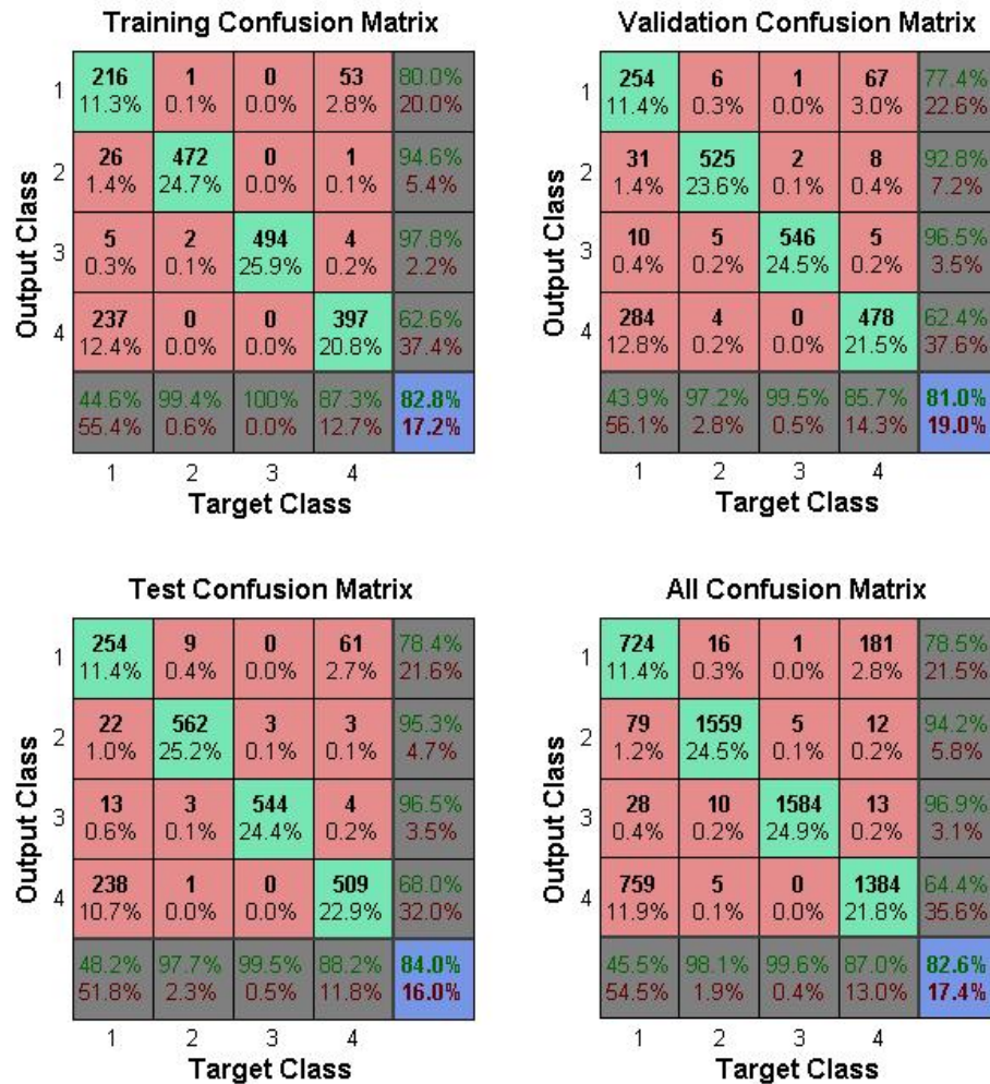
Figure 8.56: Resulting Confusion Matrix in the Flexor Muscles - S3 - Confusion matrix from the different stages of the supervised machine learning, i.e. training; validation; testing; and the summation of all the previous. The accuracy of the classification is shown for each case. For the training classification, the accuracy was 82.8% with a 17.2% of misclassification; the validation accuracy is 81% with 19% of misclassification; the test accuracy was 84% with 16% misclassification; and finally, the overall results for the flexor muscles of the forearm was 82.6% accuracy with 17.4% of misclassification.
