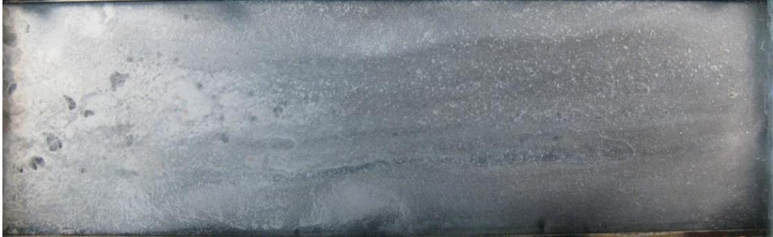
b) MICP + Colloidal Silica in the fracture after 8 cycles
