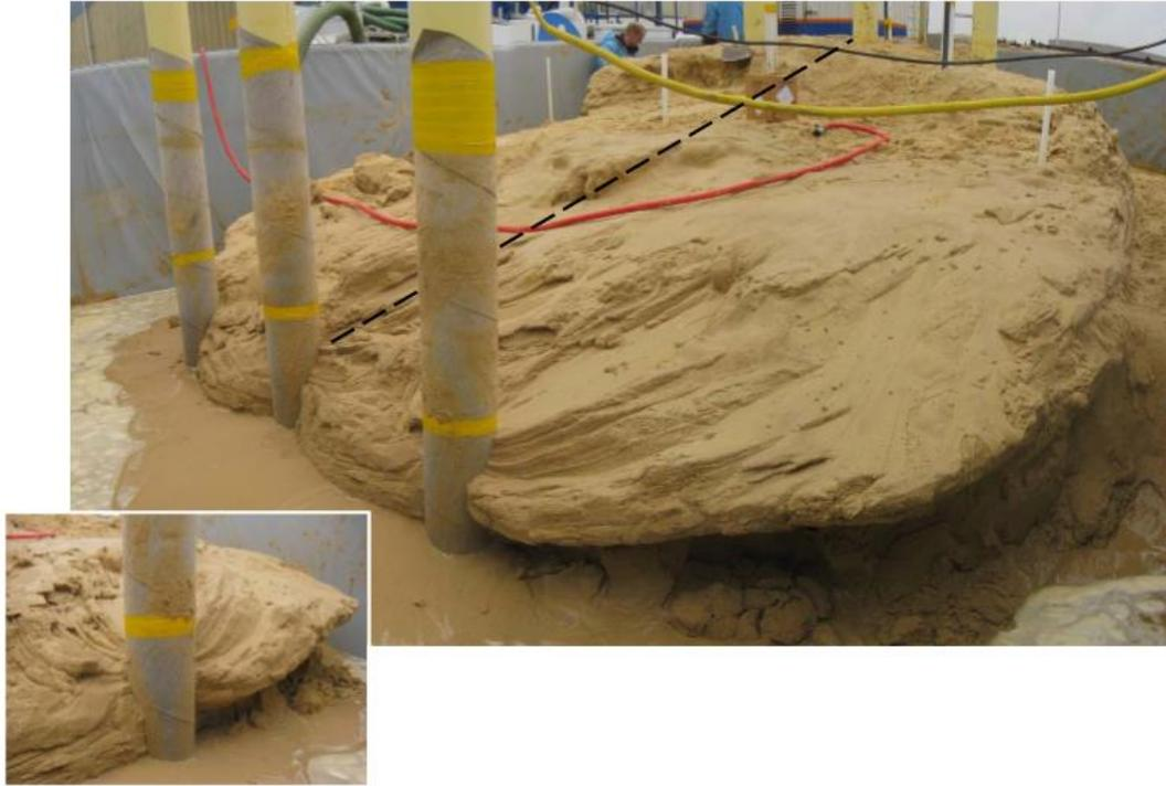
**Figure 2.3: Bacterially cemented sand approximately 43 m<sup>3</sup> in volume showing a wedge shape created by the hydrological flow from injection to extraction (columns closest in the field of view) (Van Paassen et al, 2010).**
