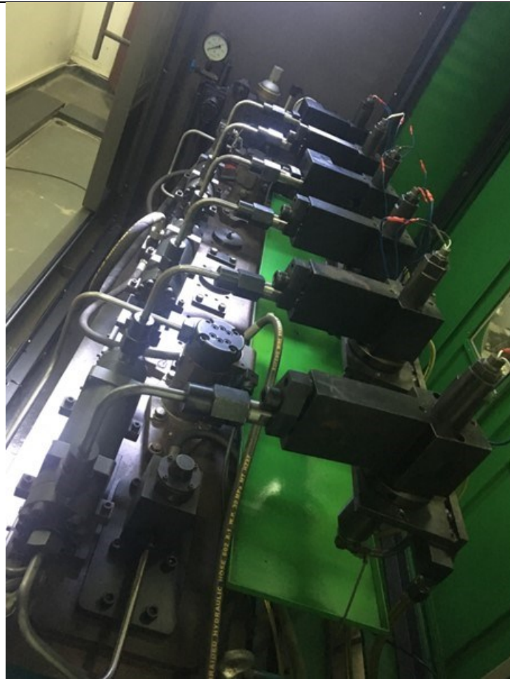
Figure 4-9 Side view of the HPCR system in the HIL test rig
