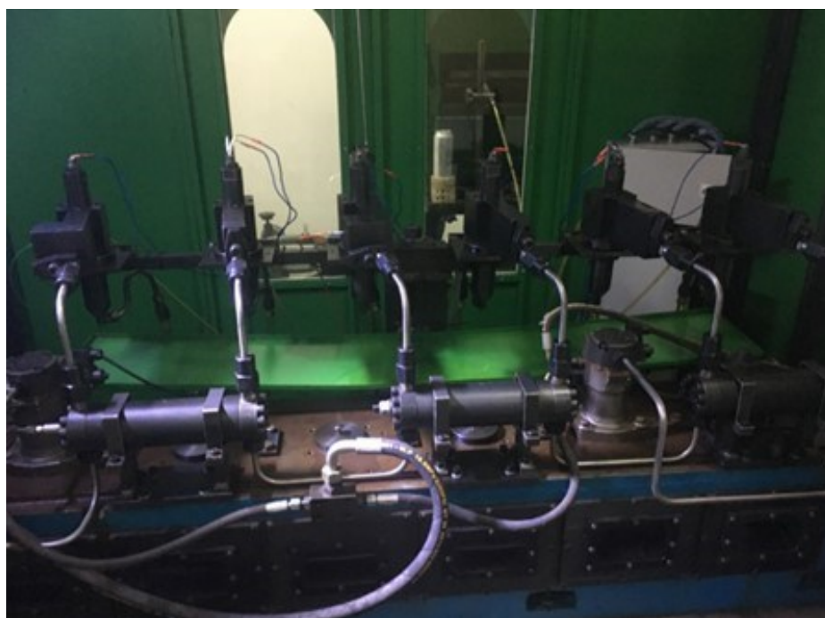
Figure 4-8 Front view of the HPCR system in the HIL test rig
