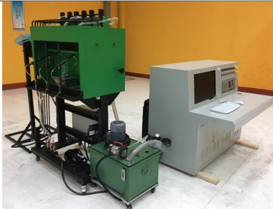
Figure 4-10 Fuel mass measuring device (left) and console desk (right)
