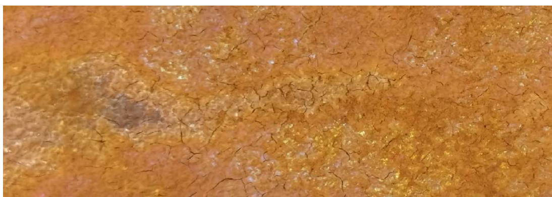
Figure 125: RF blanket is showing the structural effects of using K 2 CO 3 as a catalyst.
