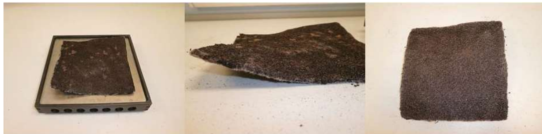
Figure 114: RF blanket prepared with a low R/C ratio (200) showing shrinkage and surface irregularities.
