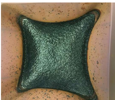
Figure 113: RF blanket fabricated using an RF sol of 40% solids, showing a high level of shrinkage after gelation and curing stages.
