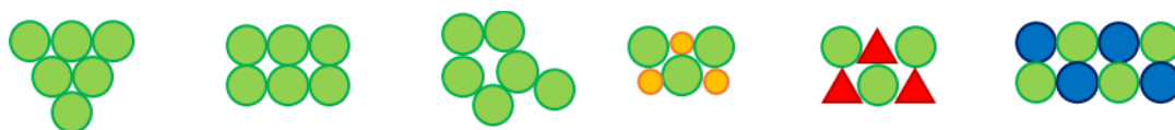
Figure 5. Schematic of various solid-state forms (from left to right): polymorph form I, polymorph form II, amorphous, solvate, salt and co-crystal.
