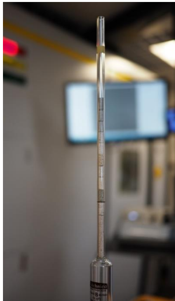
Figure 2-23: the 10 core cylinders were stack in a glass tube for X-ray \mu CT analysis.
