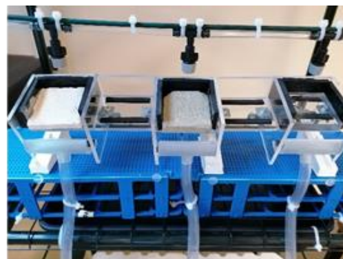
Figure 2-16: set-up of the trial test, with the pump connected to the three nozzles. Two samples and 1 procedural blank were exposed.
