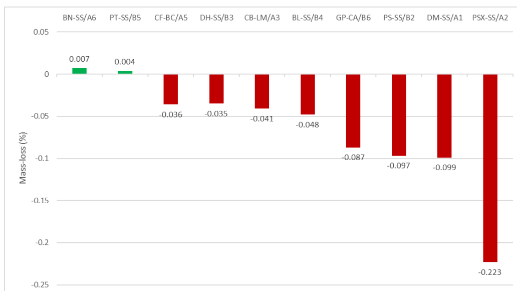
Figure 6-17: mass loss experienced by the stone types of test-set 2.
