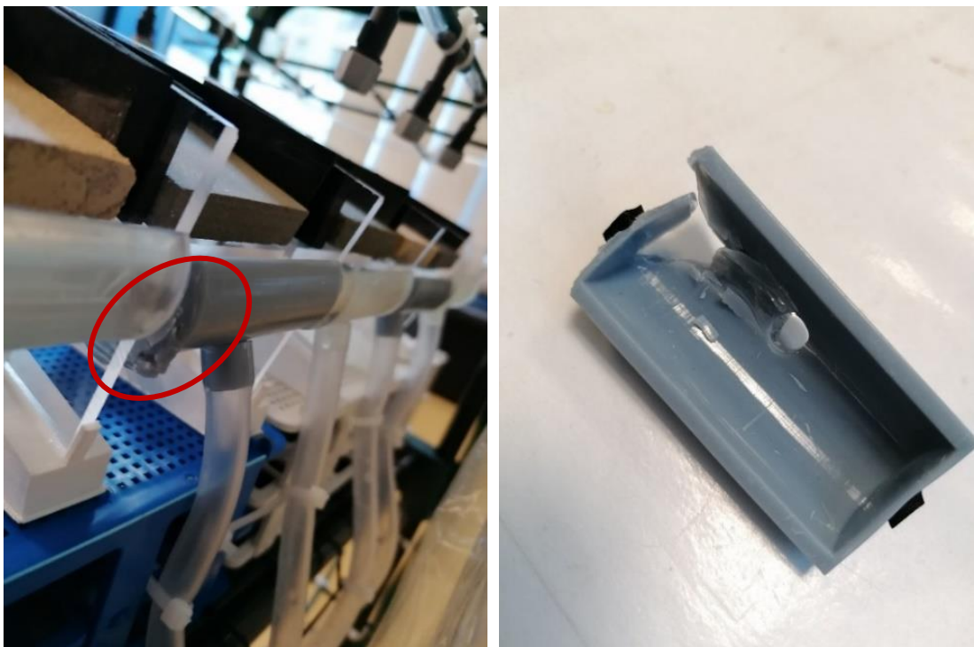
Figure 2-18: detail of the exposure apparatus showing the failure of one of the coloured resin gutters.
