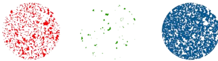
Figure 10-12: information acquired from image processing techniques on total porosity (P), carbonate minerals (C) and quartz (Q) for DM-SS.
